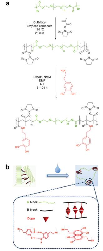
Fig. 1 Design and processing of precursor. (a) Schematic showing the synthesis of poly(NHSMA)-b-PEG-b-poly(NHSMA) (ABA-Dopa(-)) and poly(NHSMA)-b-PEG-b-poly(NHSMA)-Dopa (ABA-Dopa(+)) triblock copolymers. (b) Schematic illustration of polymer processing to create the hydrated ABA-Dopa(+) network.
