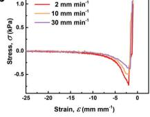
Fig. 4 Wet adhesion properties of ABA triblock copolymer networks. (a) Stress-strain curves extracted from force-distance curves between glass probes and substrates composed of networks prepared from ABA-Dopa(-) and ABA-Dopa(+) polymers. (b) Stress-strain curves for ABA-Dopa(+) networks performed at different retraction rates.
