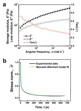
Fig. 2 Viscoelastic properties of ABA-Dopa(+) networks comparison to linear viscoelastic models. (a) Storage (E') and loss (E'') modulus are plotted as a function of angular frequency obtained from tensile oscillatory sweeps ( $\varepsilon$  = 0.5%;  $\omega$  = 0.1–100 rad s<sup>-1</sup>). (b) Plots of stress relaxation curves for both experimental data and fitting curve using Maxwell-Wiechert model (inset).
