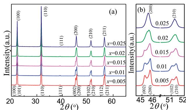
Fig. 3 Room-temperature XRD patterns of  $(1 - x)(0.96\text{KNNT} - 0.04\text{BNKZ}) - x\text{CZ}$  ceramics (a)  $2\theta = 20 - 65^\circ$ . (b)  $2\theta = 44 - 53^\circ$ .
