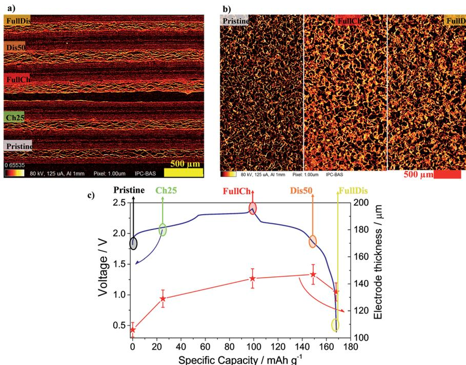
**Fig. 2** (a) CT cross-sections of four charged electrodes and pristine PG. (b) In-plane cross-sections of three electrodes at different charge states. (c) The red stars indicate the average thickness of the electrodes with various degrees of intercalation (Pristine, 25Ch, FullCh, 50Dis, FullDis) in relation to the voltage profile of the Al/EMIMCl:AlCl<sub>3</sub>/PG cell galvanostatically cycled at 25 mA g<sup>-1</sup> current at 25 °C in the 0.4 to 2.4 V cut-off voltage range.
