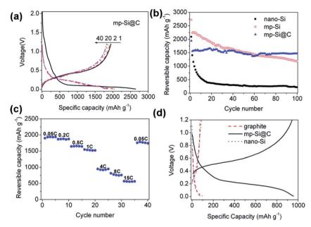
Fig. 8 (a) Voltage profile of mesoporous silicon particles with a carbon coating (mp-Si@C). (b) Cycling performance of mesoporous silicon (mp-Si), mp-Si@C and silicon nanoparticles (nano-Si). (c) Reversible capacities of mp-Si@C cycled at different current rates. (d) Voltage profiles of mp-Si, nano-Si and graphite. Figure reproduced with permission.
