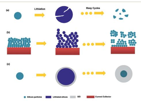
Fig. 1 Electrode failure mechanisms for silicon active material: (a) material cracking and pulverization. (b) Electrode expansion and impingement leading to isolation. (c) Continual SEI formation.<sup>13</sup> Image reproduced with permission.
