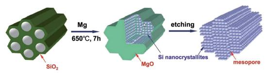
Fig. 5 Illustration of the magnesiothermic reduction process to produce porous silicon from silica.<sup>39</sup> Figure reproduced with permission.
