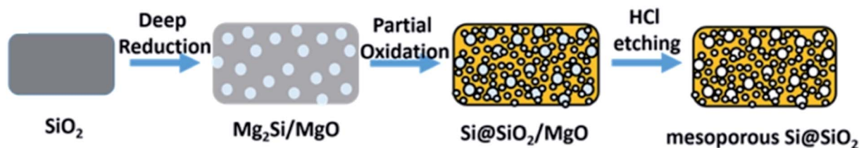
Fig. 7 Schematic illustration of the deep reduction and partial oxidation process. Reprinted with permission from ref. 63. Copyright (2016) American Chemical Society.
