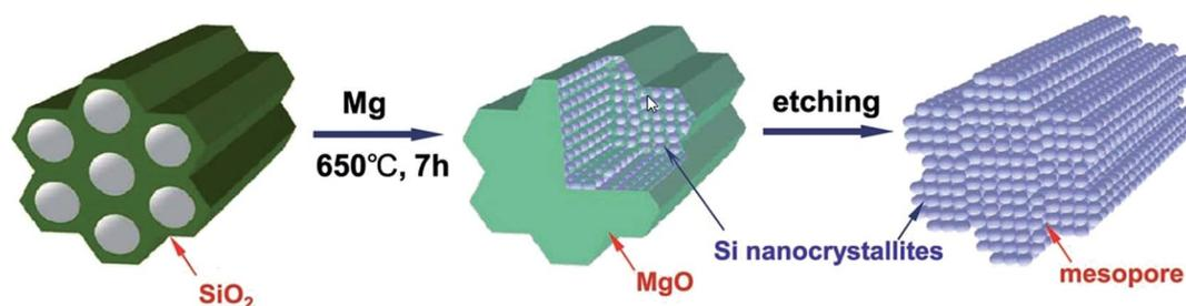
Fig. 5 Illustration of the magnesiothermic reduction process to produce porous silicon from silica.<sup>39</sup> Figure reproduced with permission.
