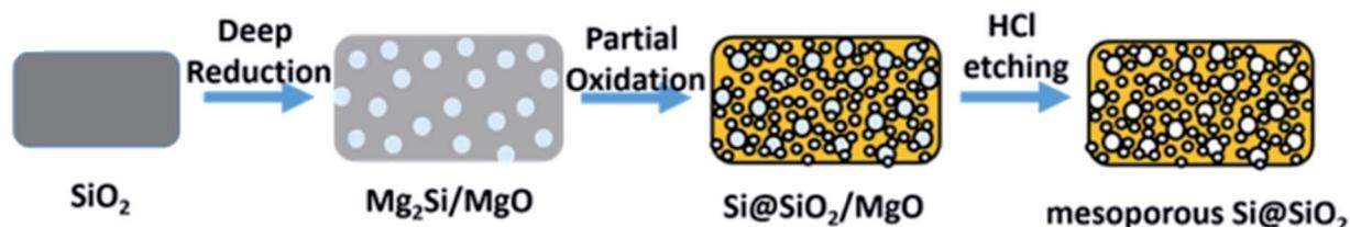
Fig. 7 Schematic illustration of the deep reduction and partial oxidation process. Reprinted with permission from ref. 63. Copyright (2016) American Chemical Society.
