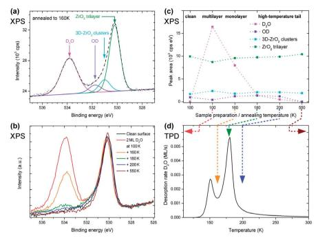
Fig. 2 XPS of  $D_2O$  on  $ZrO_2/Pt_3Zr$ . (a) O 1s region with 2 ML  $D_2O$  deposited at 100 K, then annealed to 160 K to remove the multilayer. (b) Comparison of spectra before and after  $D_2O$  adsorption, and after additional annealing steps. All XPS spectra were taken at 100 K. (c) Peak areas of the spectra in (b) for the peaks assigned to  $D_2O$ , OD, 3D  $ZrO_2$  clusters, and the  $ZrO_2$  trilayer. (d) TPD measurement (1.54 ML) for comparison with the XPS results in (b, c).
