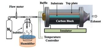
Fig. 1 The schematic illustration of aerosol assisted chemical vapour deposition (AACVD) apparatus.
