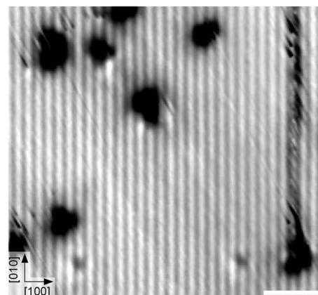
Fig. 4 STM image after dosing 0.025 L O<sub>2</sub> at 110 K. The molecules appear as streaks across point defects. STM parameters: V<sub>sample</sub> = +1.0 V, I<sub>tunnel</sub> = 0.1 nA, T<sub>sample</sub> = 78 K; fast scan direction is 58° clockwise from horizontal. The scale bar corresponds to 3 nm.
