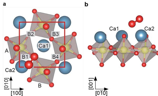
**Fig. 2** DFT model of  $\text{O}_2^-$  adsorbed on  $\text{Ca}_3\text{Ru}_2\text{O}_7$ . (a) Top view and (b) side view of the vdW-DFT model for  $\text{O}_2^-$  with  $E_{\text{ads}} = 1.4 \text{ eV}$ . The molecule adsorbs as a tilted superoxo species close to a Ca–Ca bridge (here B1).
