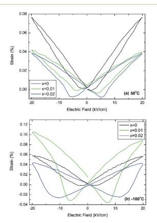
Fig. 4 Electric-field induced strain at (a) 50 °C and (b) -100 °C for (1 - x)BaTiO<sub>3</sub> -xBiYbO<sub>3</sub> ceramics.
