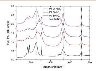
Fig. 9 Composition-dependent Raman spectra of BiYbO3 and LaYbO<sub>3</sub>-doped barium titanate at −180 °C
