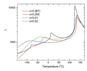
Fig. 2 Temperature dependence of the relative permittivity for (1 - x)BaTiO<sub>3</sub>-xBiYbO<sub>3</sub> ceramics measured at 10 kHz.
