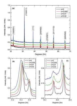
Fig. 1 (a-c) Room-temperature XRD data for  $(1 - x)BaTiO_3 - xBiYbO_3$ ceramics in the  $0 \le x \le 0.02$  range
