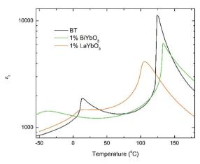
Fig. 6 Temperature dependence of the relative permittivity for (1 - x)BaTiO<sub>3</sub>-xBiYbO<sub>3</sub> and (1 - x)BaTiO<sub>3</sub>-xLaYbO<sub>3</sub> ceramics in the  $0 \le x \le$ 0.01 range.
