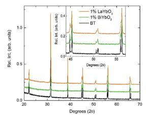
Fig. 5 Room-temperature XRD data for  $(1 - x)BaTiO_3 - xBiYbO_3$  and  $(1 - x)BaTiO_3 - xLaYbO_3$  ceramics in the  $0 \le x \le 0.01$  range.
