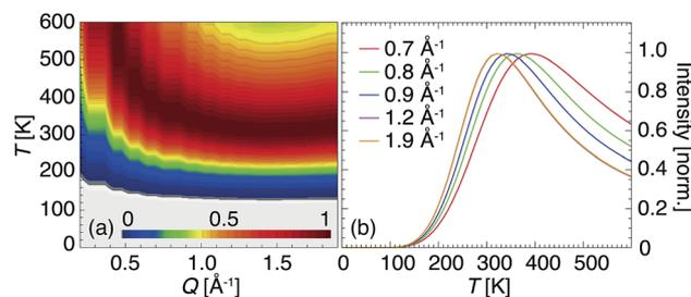
Fig. 5 IFWS signal computed for the  $Q$  range accessible on IN16B. Contrast plot of the IFWS response highlighting the maximum dependence on  $Q$  and  $T$  up to 600 K (a). Selected profiles at  $Q$  specific for the present experiment plotted in Fig. 4 (b).
