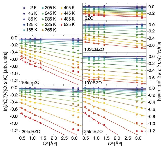
Fig. 1 Relative elastic intensities  $\ln[I(Q, T)/I(Q, 2 \text{ K})]$  measured in the EFWS mode. Results of fits with a linear dependence upon  $Q^2$  up to 1.4  $\text{\AA}^{-2}$  (In-doped series) or 1.9  $\text{\AA}^{-2}$  (BZO, 10Sc:BZO, and 10Y:BZO) are plotted as lines.
