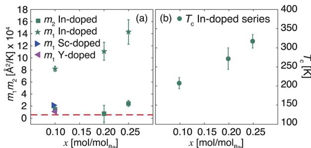
Fig. 3 Parameters  $m_1$ ,  $m_2$  (a) and  $T_c$  (b) derived from fits of eqn (3) to  $\Delta U_{\text{iso}}(Q, T)$  reported in Fig. 2. The dashed red line in panel (a) highlights the  $m_1$  value for the undoped material (BZO). When not displayed, errors are within the symbols or the thickness of the line.
