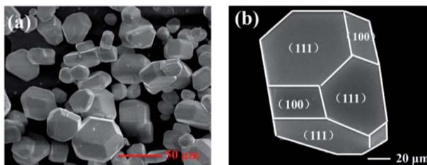
**Fig. 2** (a) Typical SEM images of Cs<sub>2</sub>AgSbCl<sub>6</sub> crystals, (b) one representative microcrystal showing different facets.
