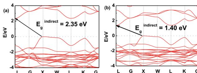
**Fig. 4** Electronic band structure of the double-perovskite Cs<sub>2</sub>AgSbCl<sub>6</sub> by HSE (a) and PBE (b) approaches.
