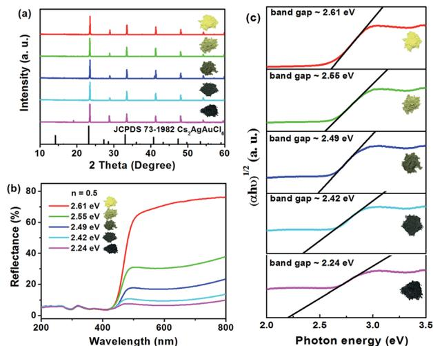
**Fig. 3** Powder XRD patterns (a), UV-vis diffuse reflectance spectra (b), and Tauc plots (c) of different as-prepared Cs<sub>2</sub>AgSbCl<sub>6</sub> obtained by using different amounts of HCl (0.5, 0.75, 1.0, 1.25 and 1.5 mL) with variable visible light absorbance.
