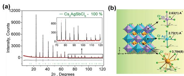
Fig. 1 (a) Observed (black), calculated (red), and difference (gray) XRD profiles for the refinement of the  $\text{Cs}_2\text{AgSbCl}_6$  sample using the Rietveld method. (b) Crystal structure of  $\text{Cs}_2\text{AgSbCl}_6$  and coordination environments for  $\text{Sb}^{5+}$ ,  $\text{Ag}^+$ , and  $\text{Cl}^-$  are given.
