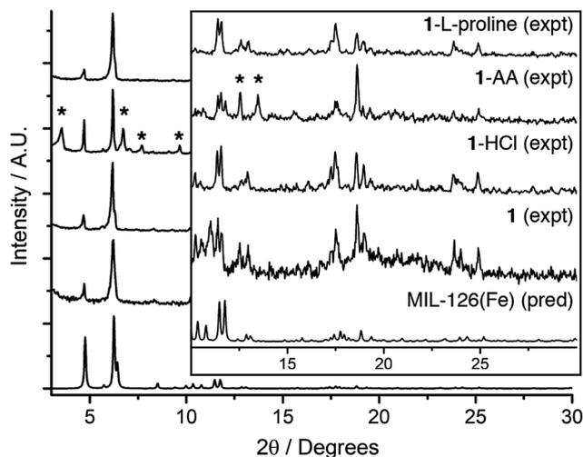
Fig. 2 Stacked PXRD patterns of the Sc-bpdc MOF, **1**, prepared with different modulators, compared with the predicted pattern of MIL-126(Fe) (CCDC code MIBMER).<sup>37</sup>
