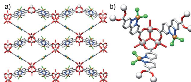
Fig. 5 The solid-state structure of **2-CuCl<sub>2</sub>** showing (a) the packing arrangement of metallated bpydc ligands, and (b) the ordering of metallation around the  $Sc_3O$  SBU. H atoms removed for clarity, all partially occupied  $CuCl_2$  positions displayed; C atoms grey, O atoms red, N atoms blue, Cl atoms green spheres, Sc atoms silver spheres; Cu atoms bronze spheres.
