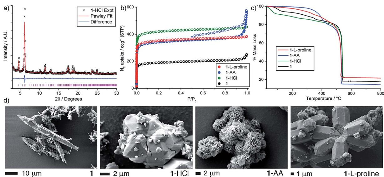
Fig. 3 (a) Pawley fitting of PXRD data for **1**-HCl ( $a = 21.8044$ ,  $b = c = 35.3996$  Å;  $\alpha = \beta = \gamma = 90^\circ$ ,  $R_{wp} = 8.07\%$ ). (b) N<sub>2</sub> uptake isotherms (77 K) for the modulated samples of **1**. Closed circles indicate adsorption, empty circles desorption. (c) Thermogravimetric analysis (TGA) profiles of the modulated samples of **1**. (d) SEM images of the modulated samples of **1**.
