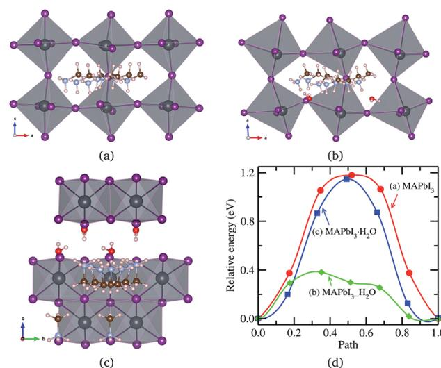
Fig. 5 MA<sup>+</sup> ion migration in (a) pseudo-cubic MAPbI<sub>3</sub>, (b) water intercalated phase MAPbI<sub>3</sub>·H<sub>2</sub>O and (c) monohydrated phase MAPbI<sub>3</sub>·H<sub>2</sub>O, and (d) corresponding activation energy profile.
