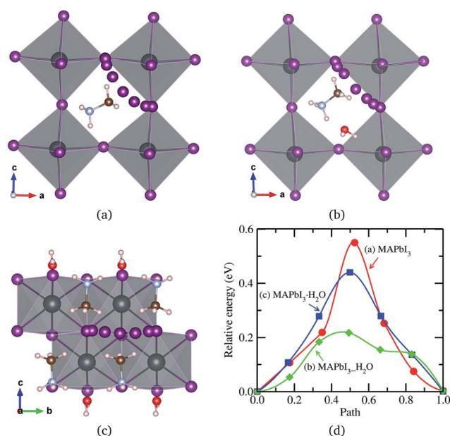
Fig. 4 I<sup>-</sup> ion migrations in (a) pseudo-cubic MAPbI<sub>3</sub>, (b) water intercalated phase MAPbI<sub>3</sub>·H<sub>2</sub>O and (c) monohydrated phase MAPbI<sub>3</sub>·H<sub>2</sub>O, and (d) corresponding activation energy profile. All the atoms are allowed to relax during migration, resulting in slight distortion of PbI<sub>6</sub> octahedra.
