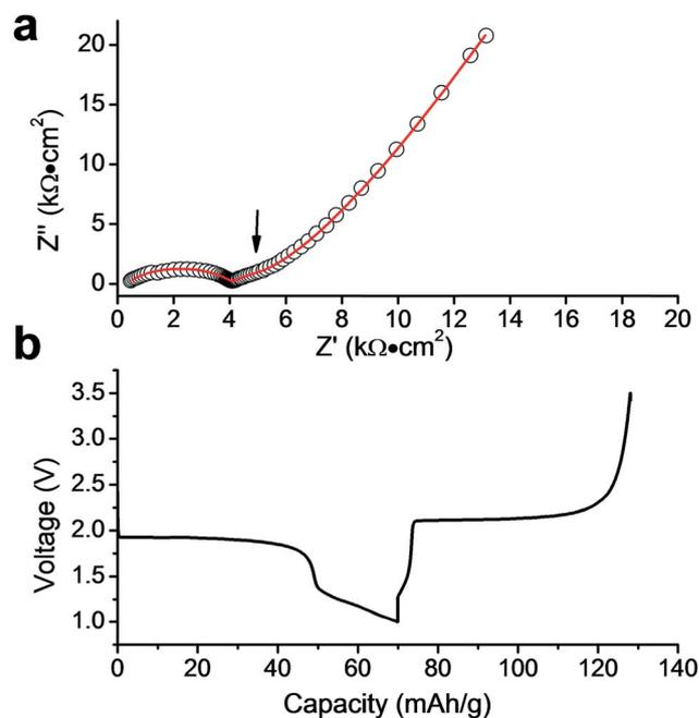
Fig. 9 (a) The impedance spectrum collected from the Li/LZP/LTP cell (LTP pellet thickness  $\sim 0.9$  mm) at 50 °C; the arrow indicates an intermediate-frequency semicircle assigned to the LTP/LTP interfacial resistance. (b) Discharge/charge profile of the Li/LZP/LTP cell at 50 °C and  $6 \mu\text{A cm}^{-2}$ .
