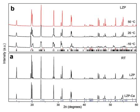
Fig. 1 (a) XRD patterns of LZP-1100 and LZP-Ca prepared by quenching; the markers (blue) are for the rhombohedral LZP phase. (b) XRD patterns of LZP-1100 at selected temperatures; the top markers (red) are for the rhombohedral phase and the bottom markers (black) are for the triclinic phase.
