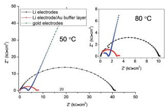
Fig. 4 Impedance plots of LZP-1100 using different electrodes at 50  $^{\circ}$ C (pellet thickness = 1.5 mm). The inset shows the spectra collected at 80  $^{\circ}$ C.
