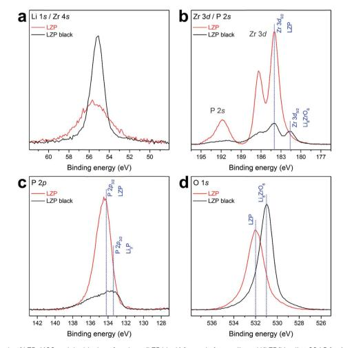
Fig. 7 XPS core levels of LZP-1100 and the black surface layer (LZP black) formed after cycling a Li/LZP/Li cell at 80 °C for 100 h, including (a) Li 1s/Zr 4s, (b) Zr 3d/P 2s, (c) P 2p, and (d) O 1s.
