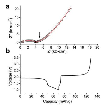
Fig. 9 (a) The impedance spectrum collected from the Li/LZP/LTP cell (LZP pellet thickness  $\sim\!0.9$  mm) at 50 °C; the arrow indicates an intermediate-frequency semicircle assigned to the LTP/LZP interfacial resistance. (b) Discharge/charge profile of the Li/LZP/LTP cell at 50 °C and 6  $\mu\text{A}$  cm $^{-2}$ .
