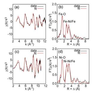
Fig. 10 EXAFS spectra with fits and their Fourier transforms for the air-annealed x = 0.75 and (a and b) Fe and (c and d) Ni.
