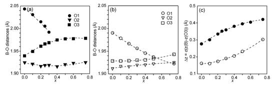
Fig. 6 (a) B-O distances in Å for the as-prepared samples, (b) B-O distances in Å for the air-annealed samples, (c)  $\Delta z = c(z(B) - z(O3))$  in Å for the as-prepared (filled circles) and air-annealed (open squares) samples.
