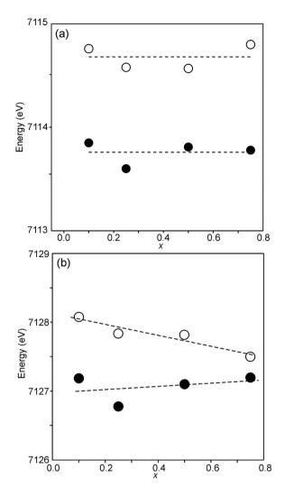
Fig. 14 (a) Centroid position of the pre-edge peak and (b) position of the main edge peak in the Fe K-edge XANES spectra. Filled circles denote the as-prepared samples and open circles denote the airannealed samples
