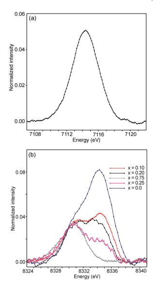
Fig. 15 (a) Fe pre-edge peak for the as-prepared x = 0.1 and (b) Ni preedge peaks for the as-prepared samples.
