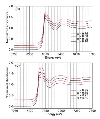
Fig. 11 XANES K-edge spectra of the as-prepared samples; (a) Ni and
