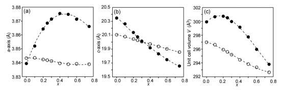
Fig. 7 Unit-cell parameters a and c in Å and unit cell volume of the as-prepared (solid circles) and air-annealed (open circles)  $Sr_{3-x}Y_xFe_{1.25}Ni_{0.75}O_{7-\delta}$
