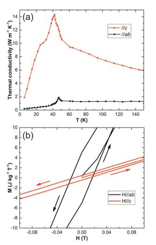
Fig. 4 (a) Variation of thermal conductivity with temperature for gaudefroyite along c (upper plot) and in the ab plane (lower plot). (b) Magnetic hysteresis of gaudefroyite at 1.8 K.
