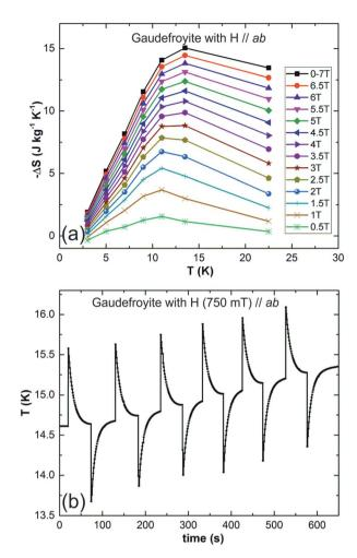
**Fig. 3** (a) Entropy changes as a function of temperature for fields of 0.5 to 7 T for gaudefroyite and (b) temperature change of gaudefroyite on applying and removing a field of 750 mT.
