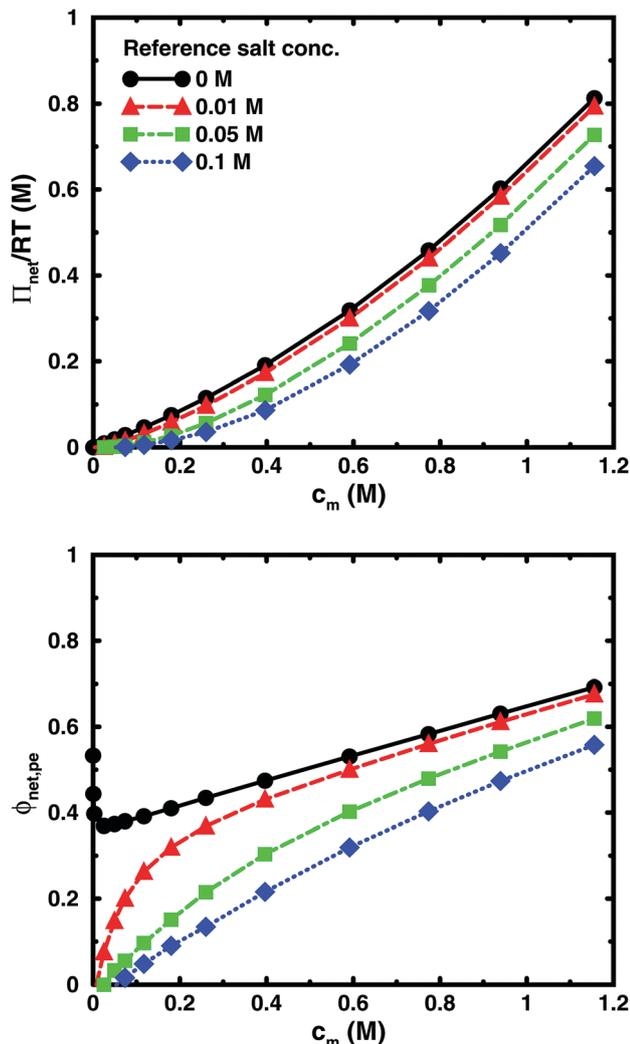
Fig. 12 The net osmotic pressure (top) and the corresponding osmotic coefficient (bottom) as a function of monomer concentration for 64mers ( $b = 4.5 \text{ \AA}$ ,  $\alpha = 1$ ) with different concentrations of the reference salt solution:  $c_s = 0 \text{ M}$  (circles, black solid lines),  $0.01 \text{ M}$  (triangles, red dashed lines),  $0.05$  (squares, green dot-dashed lines), and  $0.1 \text{ M}$  (diamonds, blue dotted lines).
