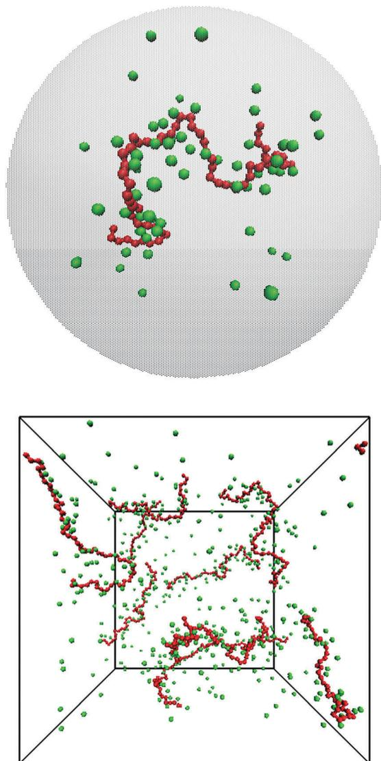
**Fig. 1** In this work, polyelectrolyte solutions are typically simulated as either a single freely jointed chain of charged hard spheres (red) with neutralising counterions (green) confined in a spherical cell with radius  $R_{\text{cell}}$  (top) or eight such polyelectrolytes in a cubic box with periodic boundary conditions (bottom). The examples show snapshots of fully charged ( $\alpha = 1.0$ ) salt-free 64mers with bond length  $b = 4.5$  Å and a monomer concentration of 0.074 M.
