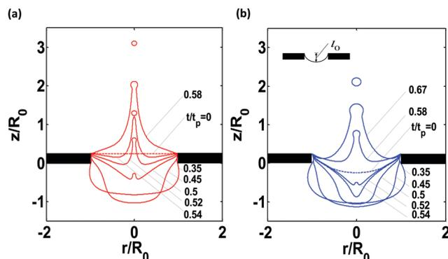
Fig. 7 Jetting simulation of silicone oil 10 cSt from the 2 mm diameter nozzle with a fixed piston velocity amplitude of  $1.97 \text{ mm s}^{-1}$  to show the influence of the initial meniscus form. (a) Plane meniscus and (b) concave meniscus.
