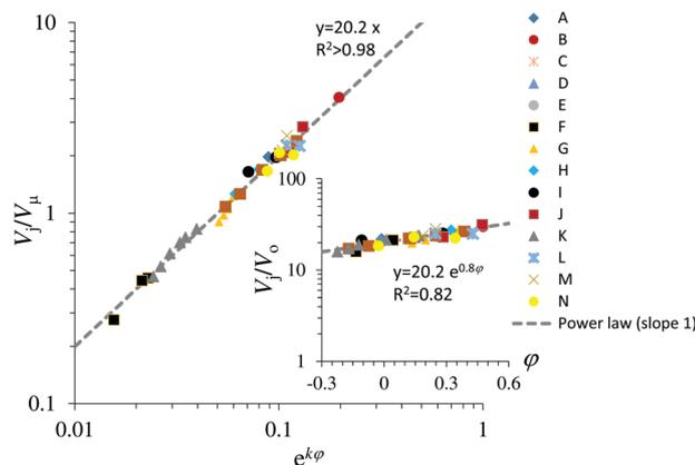
Fig. 13 Jet velocity  $V_j$  made dimensionless with either  $V_0 = R_0/t_p$  (inset) or  $V_\mu$ , showing the agreement of the scaling proposed. The open symbols represent experimental data while the closed symbols represent numerical data.
