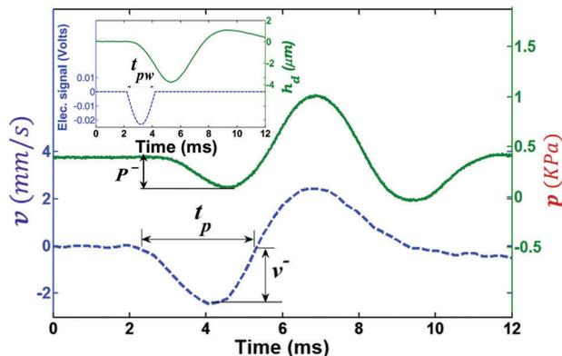
Fig. 4 Driving electrical waveform pulse and its corresponding piston displacement  $h_d$  (top left figure), piston velocity  $v$  and the pressure inside the reservoir  $p$  (main figure).  $t_{pw}$  and  $t_p$  are the pulse widths in terms of the electrical signal and velocity, respectively. Our results show that the driving pulse width and the time for cavity collapse occur at the same order of magnitude, typically a few milliseconds. Dataset available in the ESI.†<sup>40</sup>
