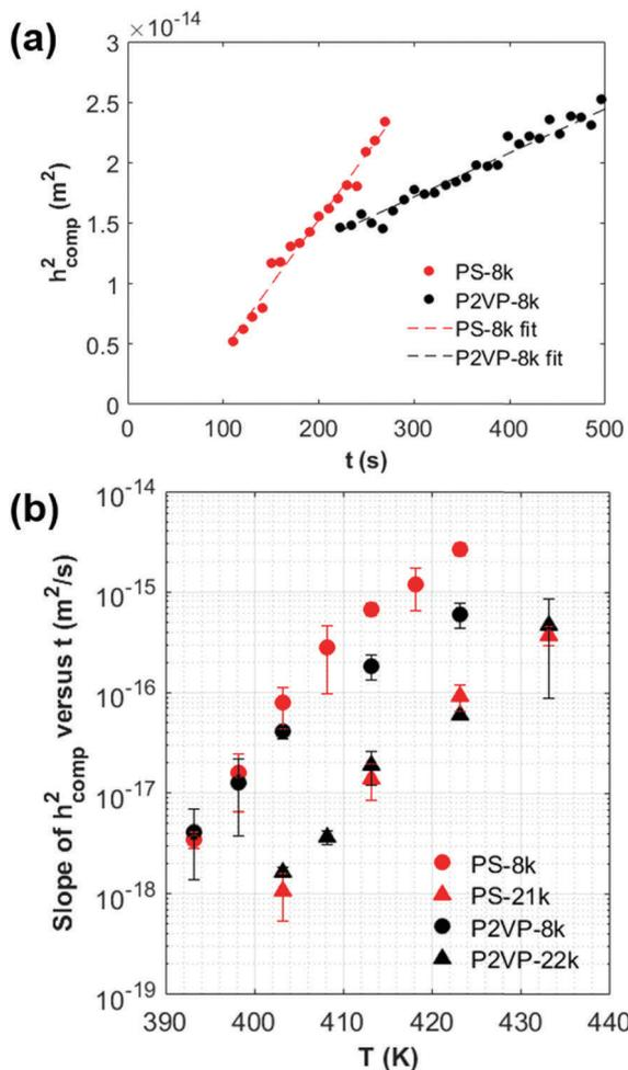
Fig. 3 (a) The composite layer thickness squared,  $h_{\text{comp}}^2$  of PS-8k and P2VP-8k composite versus annealing time,  $t$ , when the bilayer films are annealed at 403 K, shows a linear fit and agrees well with the Lucas–Washburn model. (b) The slope of  $h_{\text{comp}}^2$  versus  $t$  as a function of annealing temperature,  $T$  for PS-8k, P2VP-8k, PS-21k, and P2VP-22k.
