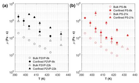
Fig. 4 Bulk and confined polymer viscosity of (a) P2VP-8k and P2VP-22k, and (b) PS-8k and PS-21k as a function of temperature. Each data point for the confined polymer viscosities is an average of at least 2 runs, and the error bar represents 1 standard deviation. The bulk viscosity values are obtained from the literature (see the ESI†).
