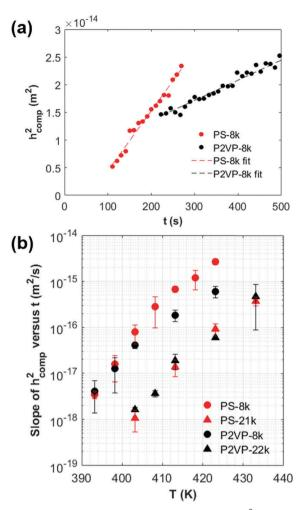
Fig. 3 (a) The composite layer thickness squared,  $h_{comp}^2$  of PS-8k and P2VP-8k composite versus annealing time, t, when the bilayer films are annealed at 403 K, shows a linear fit and agrees well with the Lucas-Washburn model. (b) The slope of  $h_{comp}^2$  versus t as a function of annealing temperature, T for PS-8k, P2VP-8k, PS-21k, and P2VP-22k.
