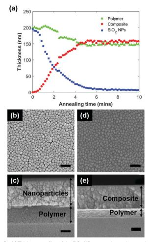
Fig. 2 (a) Thickness profiles of the SiO<sub>2</sub> NP, composite, and neat polymer layers as a function of annealing time, obtained using in situ spectroscopic ellipsometry while annealing ~200 nm SiO<sub>2</sub> NP/~200 nm PS-8k bilayer films at 403 K. The SEM images show the (b) top and (c) cross sectional views of the bilayer film before annealing, and the (d) top and (e) cross sectional views of the PINF atop a residual polymer layer after annealing. The scale bars are 100 nm.
