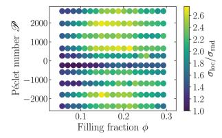
**Fig. 4** Standard deviation of local Voronoi volume  $\sigma_{\rm loc}$  compared to standard deviation  $\sigma_{\rm md}$  of a homogeneous configuration. The Péclet number  ${\mathscr P}$  as well as the global filling fraction  $\phi$  are varied. Positive Péclet numbers correspond to pusher-type and negative to puller-type swimmers.
