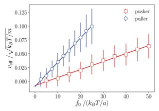
Fig. 3 Dependence of the pusher and puller velocity  $v_{\rm eff}$  on the active force  $f_0$ . Lines are linear fits to the simulated data. The observed linear dependence is evidence of the Stokes flow regime.
