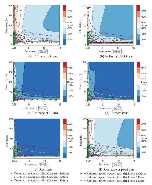
Fig. 10 Membrane properties required for cost-competitive membrane  $CO_2$  capture, including the upper bound limitation and membrane material data for cost-optimal CCRs and the six cases considered: (a) refinery FG (b) refinery LSFO (c) refinery FCC (d) cement (e) steel (f) coal power plant.
