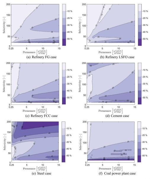
Fig. 11 Achieved cost reductions of the membrane-based  $CO_2$  capture when considering optimal CCR rather than 90% CCR for the five industrial and one power generation cases considered: (a) refinery FG (b) refinery LSFO (c) refinery FCC (d) cement (e) steel (f) coal power plant8.
