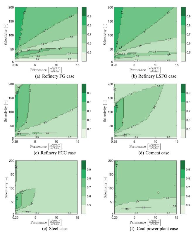
Fig. 12 Cost-optimal CCRs of the membrane-based CO<sub>2</sub> capture for the five industrial and one power generation cases considered: (a) refinery FG (b) refinery LSFO (c) refinery FCC (d) cement (e) steel (f) coal power plant.
