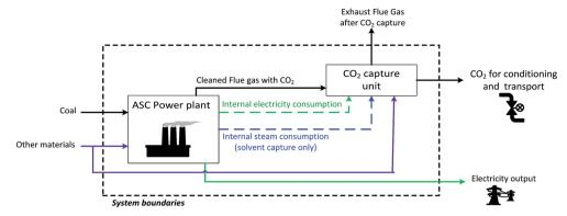
Fig. 3 Schematic view of the system boundaries for the power generation case
