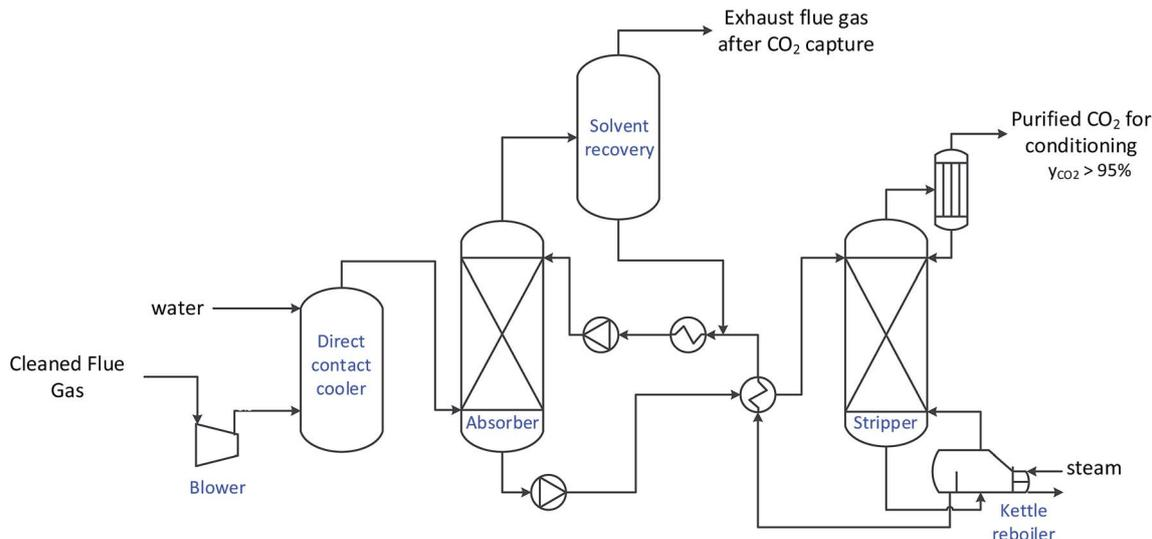
Fig. 5 Layout of the MEA-based CO<sub>2</sub> capture process.<sup>42</sup>
