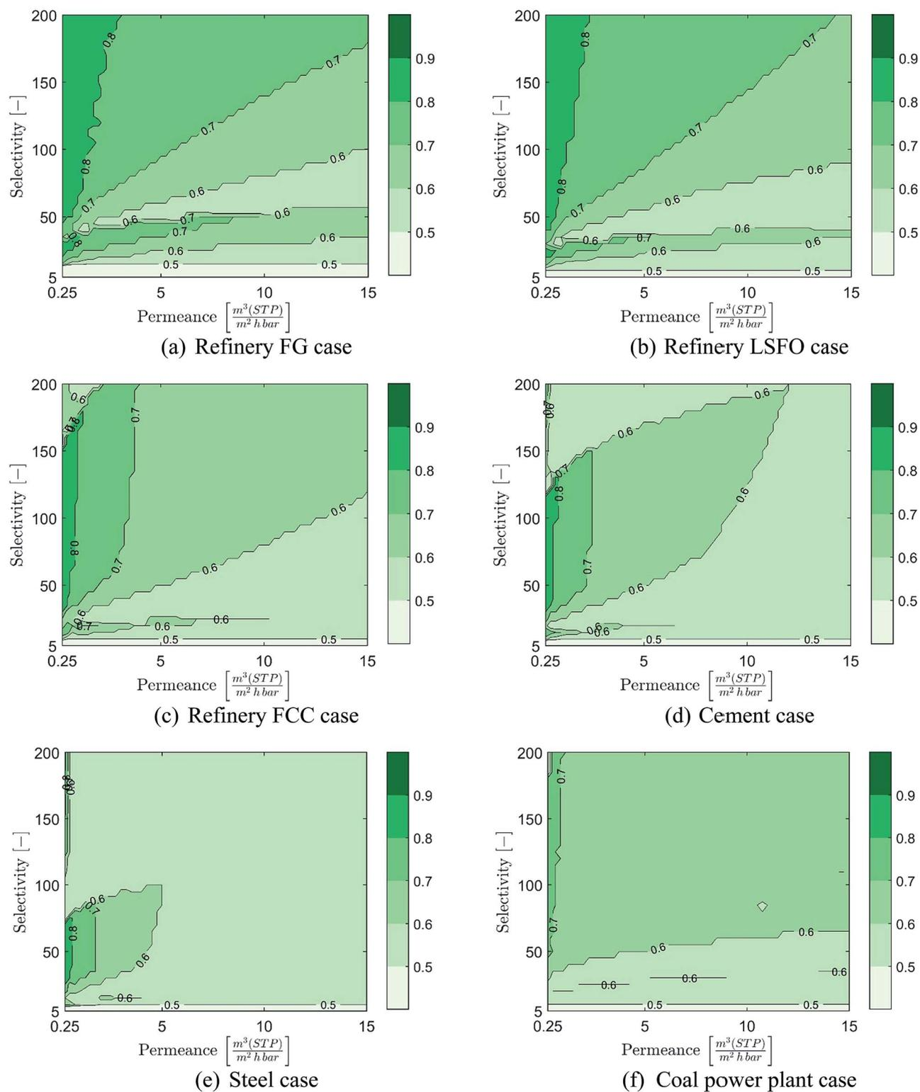
Fig. 12 Cost-optimal CCRs of the membrane-based CO<sub>2</sub> capture for the five industrial and one power generation cases considered: (a) refinery FG (b) refinery LSFO (c) refinery FCC (d) cement (e) steel (f) coal power plant.
