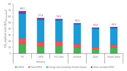
Fig. 6 Cost breakdown of the MEA-based CO<sub>2</sub> capture process.
