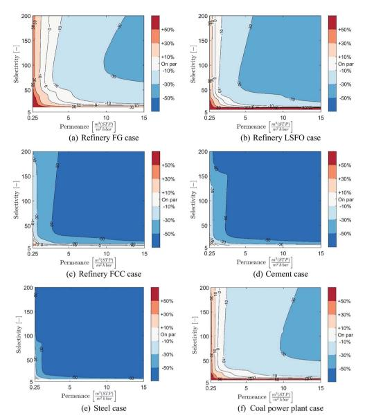
Fig. 8 Cost of membrane-based CO<sub>2</sub> capture at optimal CCRs compared to post-combustion MEA-based capture depending on the membrane properties for the six cases considered: (a) refinery FG (b) refinery LSFO (c) refinery FCC (d) cement (e) steel (f) coal power plant.
