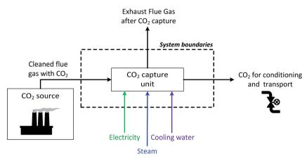
Fig. 2 Schematic view of the system boundaries for the industrial cases.§
