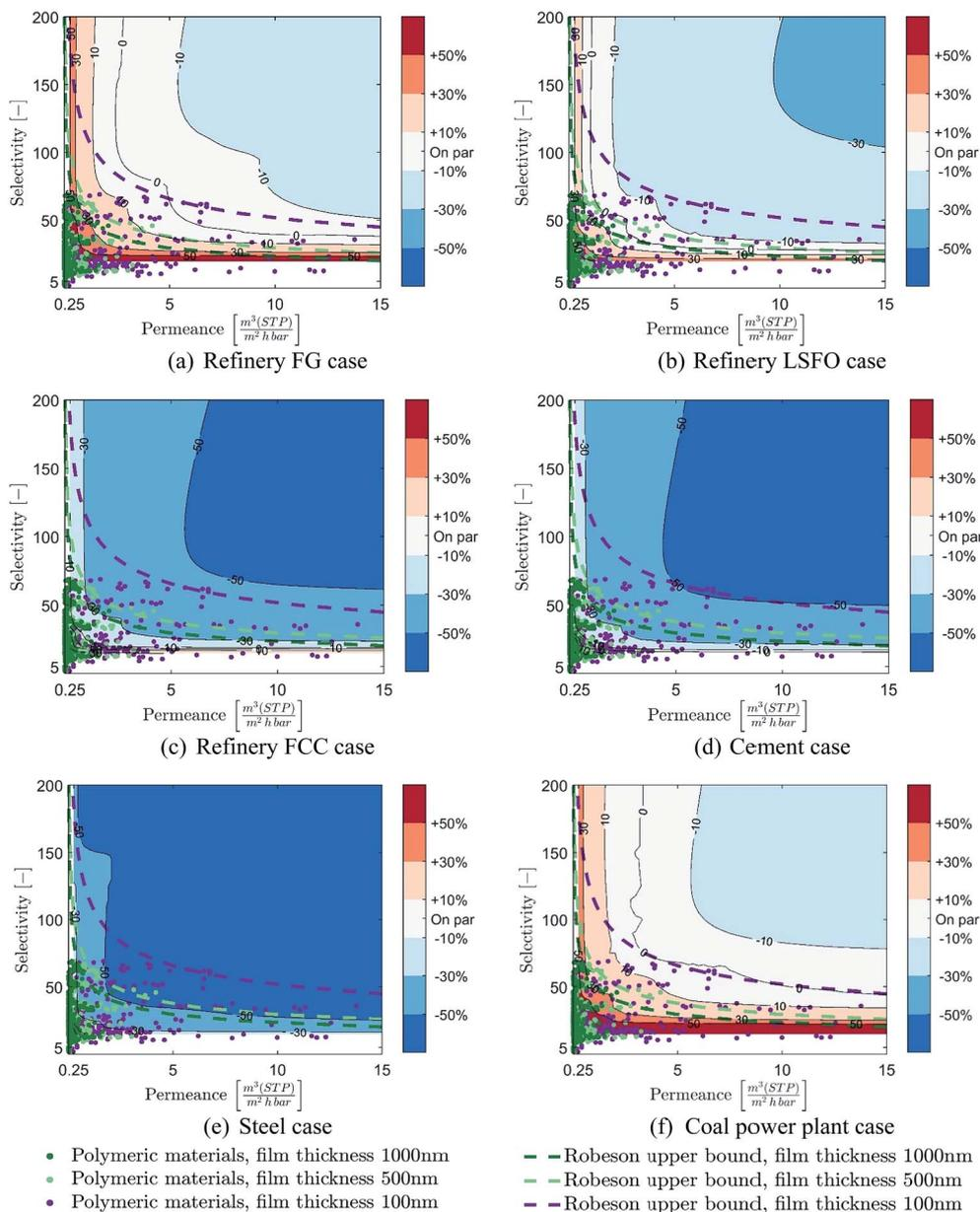
Fig. 9 Membrane properties required for cost-competitive membrane CO<sub>2</sub> capture, including the upper bound limitations and membrane material data for a 90% CCR and the six cases considered: (a) refinery FG (b) refinery LSFO (c) refinery FCC (d) cement (e) steel (f) coal power plant.
