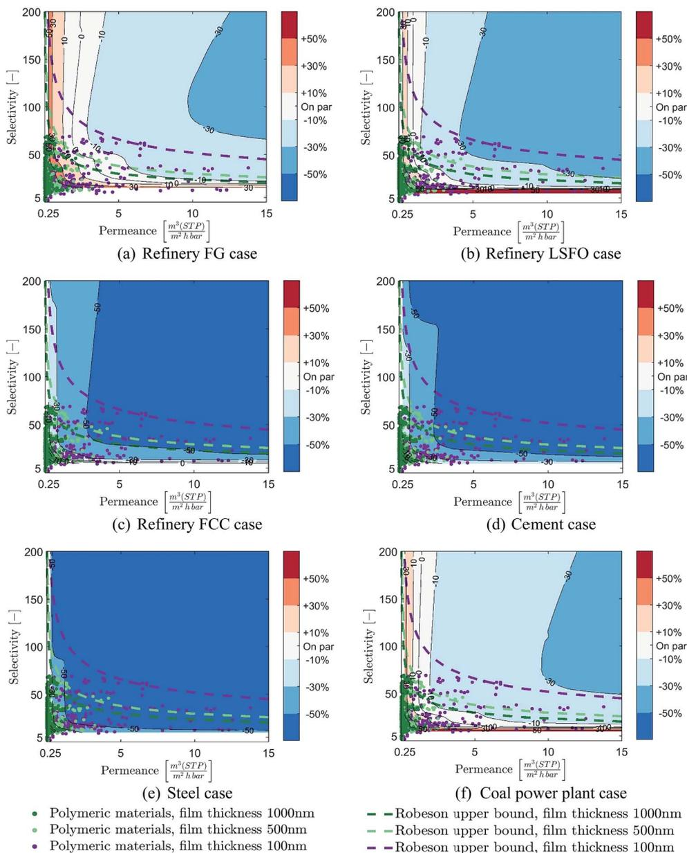
Fig. 10 Membrane properties required for cost-competitive membrane  $\text{CO}_2$  capture, including the upper bound limitation and membrane material data for cost-optimal CCRs and the six cases considered: (a) refinery FG (b) refinery LSFO (c) refinery FCC (d) cement (e) steel (f) coal power plant.
