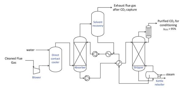
Fig. 5 Layout of the MEA-based CO<sub>2</sub> capture process.<sup>42</sup>
