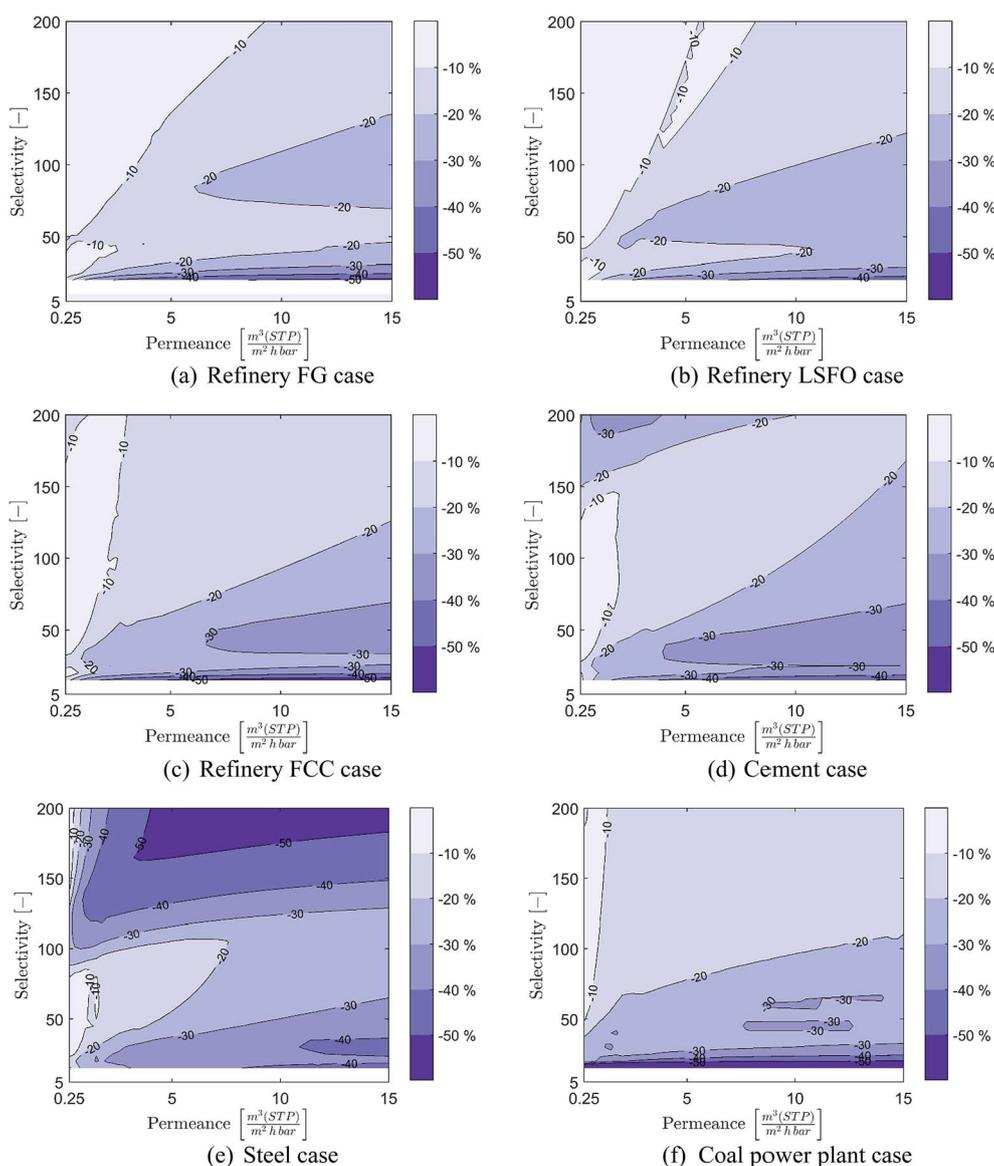
Fig. 11 Achieved cost reductions of the membrane-based CO<sub>2</sub> capture when considering optimal CCR rather than 90% CCR for the five industrial and one power generation cases considered: (a) refinery FG (b) refinery LSFO (c) refinery FCC (d) cement (e) steel (f) coal power plant8.
