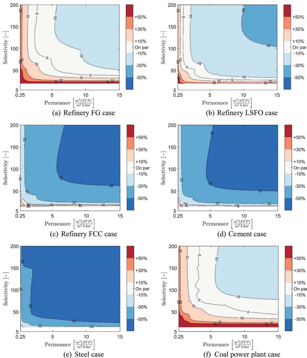
Fig. 7 Cost of membrane-based CO<sub>2</sub> capture compared to post-combustion MEA-based capture at a 90% CCR depending on the membrane properties for the six cases considered: (a) refinery FG (b) refinery LSFO (c) refinery FCC (d) cement (e) steel (f) coal power plant.
