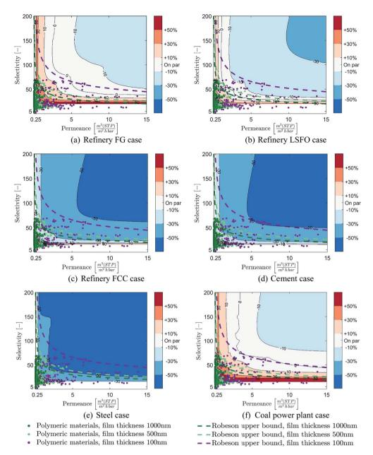
Fig. 9 Membrane properties required for cost-competitive membrane  $CO_2$  capture, including the upper bound limitations and membrane material data for a 90% CCR and the six cases considered: (a) refinery FG (b) refinery LSFO (c) refinery FCC (d) cement (e) steel (f) coal power plant.
