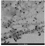
Fig. 4 TEM image of the recycled catalyst after first (left) and fifth (right) run at 50  $^{\circ}$ C. Scale bars 100 nm.
