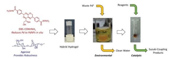
Fig. 1 Schematic of the 'waste-to-wealth' approach using DBS-CONHNH<sub>2</sub>/agarose hybrid hydrogels to remediate waste, generating PdNPs in situ and then using the resulting material to catalyse Suzuki cross-coupling reactions.
