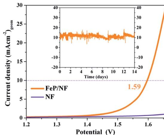
Fig. 9 LSV curves of water electrolysis for FeP||FeP on NF as anode and cathode in a two-electrode cell (sweep rate  $1\text{ mV s}^{-1}$ ) and (inset) the stability tests of corresponding electrolysis at an applied bias of 1.6 V maintaining the current of  $10\text{ mA (cm)}^{-2}$  over a period of 14 days.
