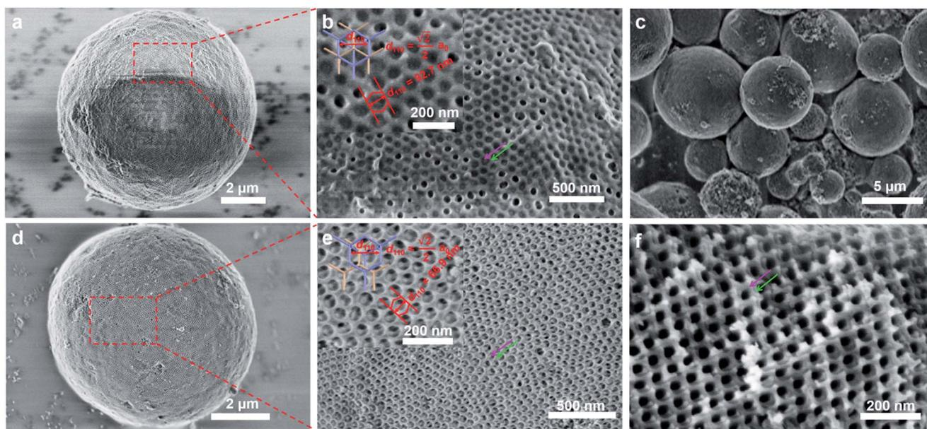
Fig. 1 FESEM images of (a, b) the as-made  $\text{Al}^{3+}$ -based gel/PEO-*b*-PMMA composite microsphere prepared by the vesicle-aggregation-assembly approach, (c–e) ordered mesoporous alumina microspheres and (f) its fragment obtained after calcination at 900 °C in air. The insets in (b) and (e) show enlarged SEM images and corresponding theoretical stick models, respectively.
