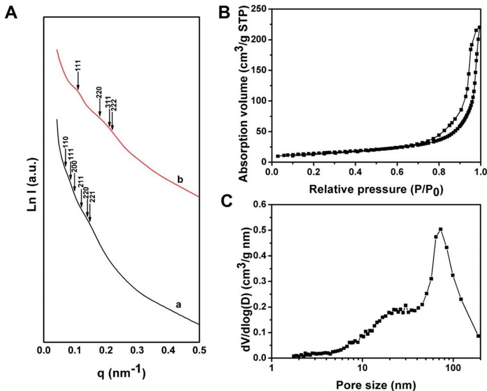
Fig. 3 (A) SAXS patterns of (a) as-made  $\text{Al}^{3+}$ -based gel/PEO-*b*-PMMA composites prepared by the vesicle-aggregation-assembly approach and (b) ordered mesoporous alumina obtained after calcination at 900 °C in air. (B) Nitrogen sorption isotherms and (C) pore size distribution of the ordered mesoporous alumina prepared by the vesicle-aggregation-assembly approach after calcination at 900 °C in air.
