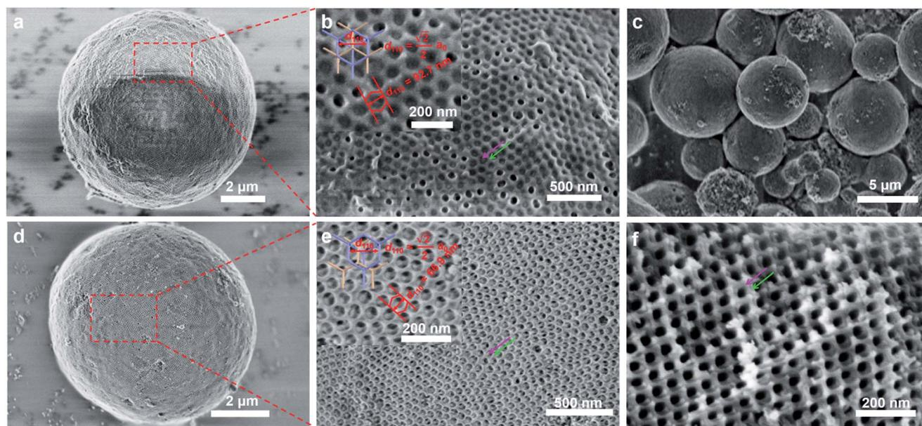
Fig. 1 FESEM images of (a, b) the as-made Al<sup>3+</sup>-based gel/PEO-*b*-PMMA composite microsphere prepared by the vesicle-aggregation-assembly approach, (c–e) ordered mesoporous alumina microspheres and (f) its fragment obtained after calcination at 900 °C in air. The insets in (b) and (e) show enlarged SEM images and corresponding theoretical stick models, respectively.
