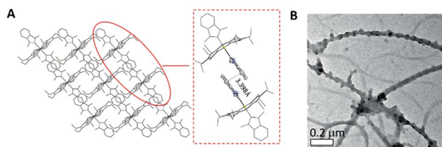
Fig. 2 (A) The crystal packing diagram of 2b viewed along the b -axis and an enlarged image of a pair of 2b molecules with an interplanar distance of 3.398 Å. (B) TEM image obtained from THF/H 2 O (1 : 90, v/v) mixture.
