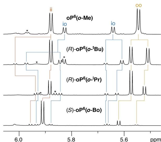
Fig. 8 Representative <sup>1</sup>H NMR spectra (850 MHz, CDCl<sub>3</sub>, 278 K) of *o*-imine *o*-phenylenes (H<sub>3e</sub> region). Signals corresponding to misfolded (AAB) conformers are marked \*.
