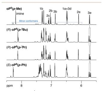
Fig. 3 Representative  $^1$ H NMR spectra (500 MHz, CDCl<sub>3</sub>, 273 K) of p-imine o-phenylenes (aromatic region). Protons H $_3$ e were used to evaluate de's. Small peaks corresponds to misfolded conformers, as confirmed by EXSY spectroscopy.
