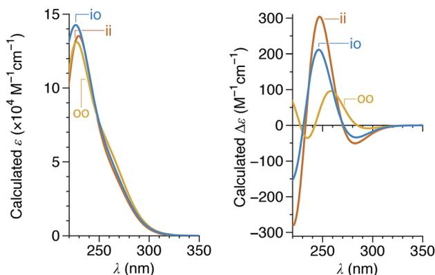
Fig. 11 Calculated UV-vis (left) and CD (right) spectra for the *ii*, *oo*, and *io* conformers of  $(M)\text{-oP}^6(\text{o-H})$  (PCM( $\text{CHCl}_3$ )/TD/CAM-B3LYP/6-31G(d,p)//PCM( $\text{CHCl}_3$ )/B97-D/TZV(2d,2p)). Spectra were simulated assuming a peak half-width at half-height of 0.333 eV.
