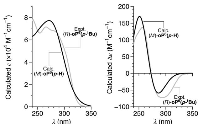
Fig. 6 Calculated UV-vis (left) and CD (right) spectra for (*M*)-**oP<sup>6</sup>(p-H)** (black) (PCM(CHCl<sub>3</sub>)/TD/CAM-B3LYP/6-31G(d,p)//PCM(CHCl<sub>3</sub>)/B97-D/TZV(2d,2p)). The calculated spectra are the Boltzmann-weighted averages of those for the three conformers in Fig. 5, obtained by assuming a peak half-width at half-height of 0.333 eV. The experimental spectra of (*R*)-**oP<sup>6</sup>(p-Bu)** are included for comparison (gray, a.u.).
