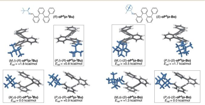
Fig. 13 Optimized M and P geometries and their relative stabilities of inward- (i) and outward-facing (o) conformers for (R)- $oP^4(o^{-t}Bu)$  (left) and (S)- $oP^4(o^{-t}Bu)$  (right) (PCM(CHCl<sub>3</sub>/B97-D/TZV(2d,2p))). Boxes indicate the favored conformers for each imine orientation.
