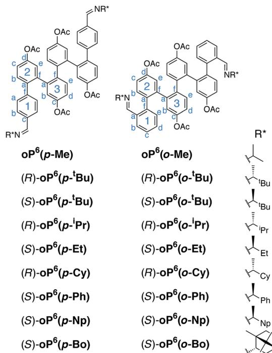
Fig. 2 *o*-Phenylene hexamers with terminal *para* and *ortho* imines (Cy = cyclohexyl, Np = 1-naphthyl, Bo = bornyl<sup>58</sup>).
