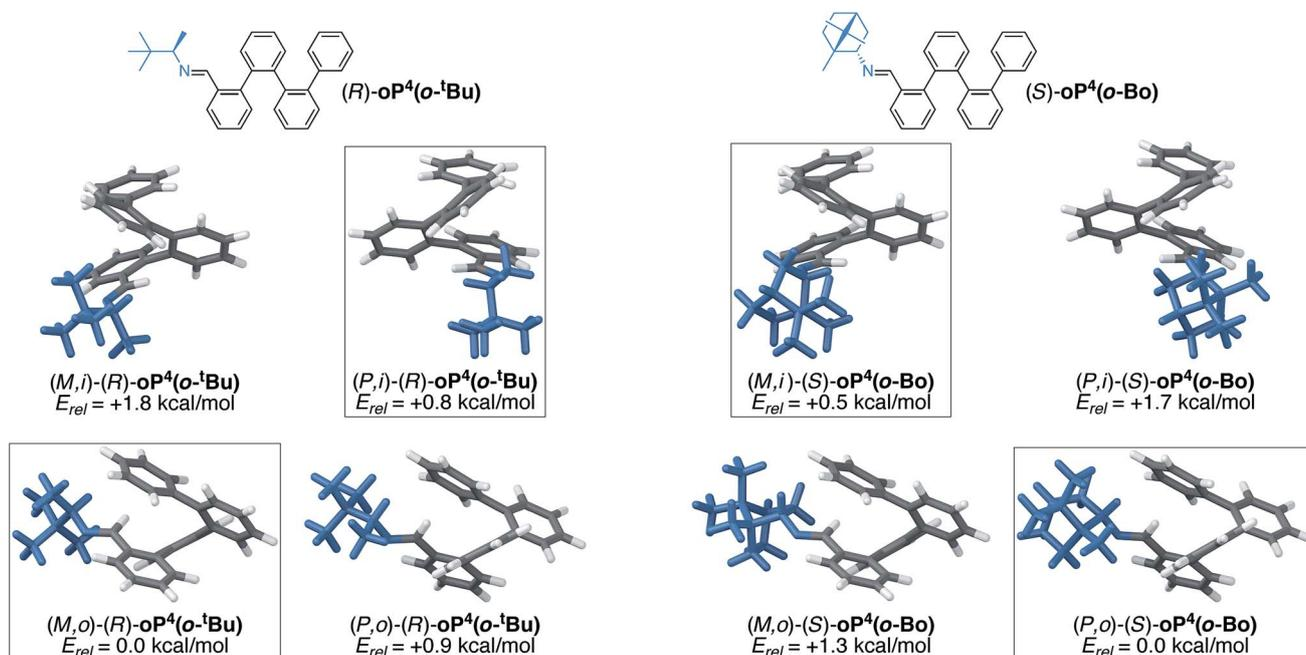
Fig. 13 Optimized *M* and *P* geometries and their relative stabilities of inward- (*i*) and outward-facing (*o*) conformers for (*R*)-**oP**<sup>4</sup>(**o-tBu**) (left) and (*S*)-**oP**<sup>4</sup>(**o-Bo**) (right) (PCM(CHCl<sub>3</sub>)/B97-D/TZV(2d,2p)). Boxes indicate the favored conformers for each imine orientation.
