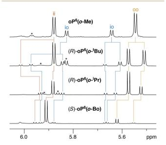
Fig. 8 Representative  $^1$ H NMR spectra (850 MHz, CDCl $_3$ , 278 K) of o-imine o-phenylenes (H $_3$ e region). Signals corresponding to misfolded (AAB) conformers are marked \*.
