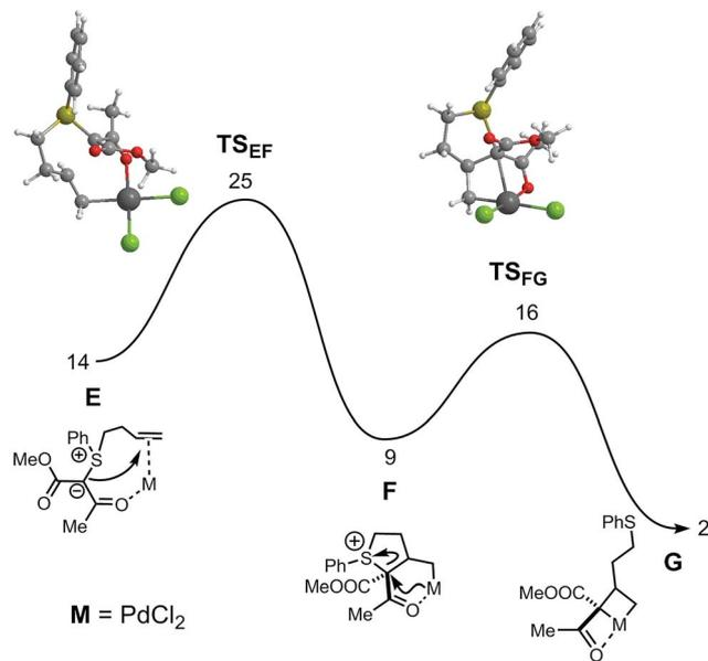
Fig. 2 Free energy profile ( $\text{kcal mol}^{-1}$ ) for the formation of the  $\text{Pd}^{\text{IV}}$  intermediate common to both reactions. Free energy values relative to the separated reactants:  $[\text{PdCl}_2(\text{MeCN})_2]$  and substrate.
