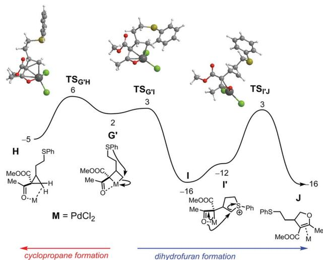
Fig. 3 Free energy profile ( $\text{kcal mol}^{-1}$ ) for the formation of dihydrofuran (right side) and for cyclopropanation (left side) from intermediate **G**. Free energy values relative to the separated reactants:  $[\text{PdCl}_2(\text{MeCN})_2]$  and substrate.
