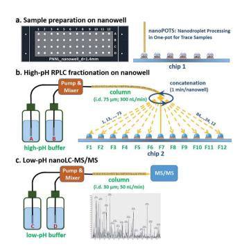
Fig. 1 Workflow for nanowell-mediated 2D LC. (a) Nanogram biological samples or small populations of cells are prepared using nanoPOTS. (b) Samples are separated using high-pH nanoflow RPLC. The eluent from the high-pH RPLC separation is concatenated into nanowells and allowed to dry. (c) Samples in each nanowell are reconstituted and collected into capillaries for subsequent low-pH nanoLC-MS/MS analysis.
