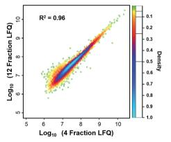
Fig. 4 Scatter plot of the proteins quantified from 12 and 4 fractions by using 50 ng HeLa digest. The Pearson coefficient for the scatter plot was calculated to be 0.96, indicating that the proteins quantified from 12 and 4 fractions had a high correlation and were very similar at the quantitative level.
