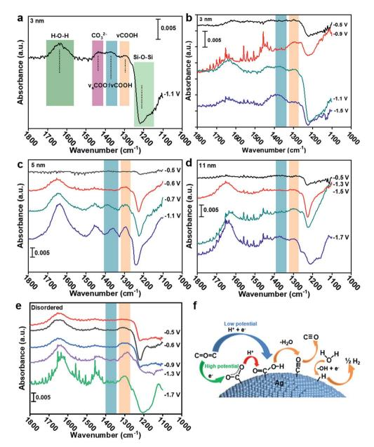
Fig. 4 (a) ATR-SEIRAS spectra of 3 nm Ag in  $CO_2$  saturated 0.1 M KCl electrolyte at -1.1 V. ATR-SEIRAS spectra of (b) 3 nm, (c) 5 nm, (d) 11 nm and (e) disordered Ag in  $CO_2$  saturated 0.1 M KCl electrolyte at different potentials. (f) Reaction mechanism for the  $CO_2$ RR and HER on the Ag surface.
