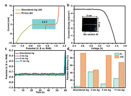
Fig. 3 (a) Performance of the disordered Ag and Pt film towards the  $CO_2RR$  and OER by linear sweep voltammetry at a scan rate of 50 mV s<sup>-1</sup> in 0.1 M KHCO<sub>3</sub>. (b) The current density-voltage characteristics of a six-section a-Si solar cell were measured under AM 1.5G illumination. (c) Cathode voltage and (d) CO FE in the PV-EC system driven by a six-section a-Si solar cell.
