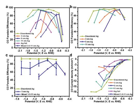
Fig. 2 CO faradaic efficiency depending on applied potential in  $CO_2$  saturated (a) 0.1 M KHCO<sub>3</sub> and (b) 0.1 M KCl, (c) CO faradaic efficiency on a simple mixture of 3-5-11 nm, disordered and 5 nm Ag in 0.1 M KHCO<sub>3</sub> with error bars. (d) CO partial current density depending on applied potential.
