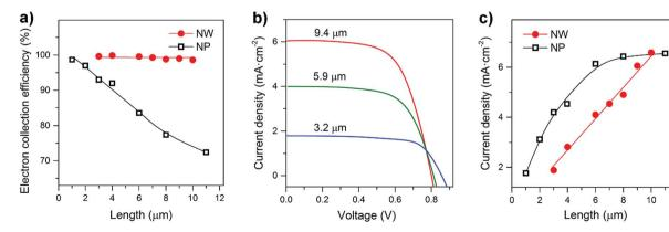
Fig. 4 Performance of the rutile  ${\rm TiO_2}$  NW and NP-based solar cells. (a) Dependence of the electron collection efficiency on the NW length and NP-film thickness. (b) Comparison of the current density-voltage characteristics of the NW-based cells under AM 1.5 illumination. (c) Dependence of current density on the NW length and NP-film thickness.
