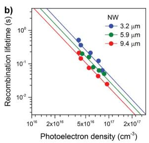
Fig. 3 Electron transport and recombination dynamics of NW-based photoelectrodes of different thicknesses. (a) Comparison of electron diffusion coefficients as a function of the photoelectron density for NW and NP based photoelectrodes. (b) Comparison of recombination lifetimes as a function of photoelectron density for NW based photoelectrodes.
