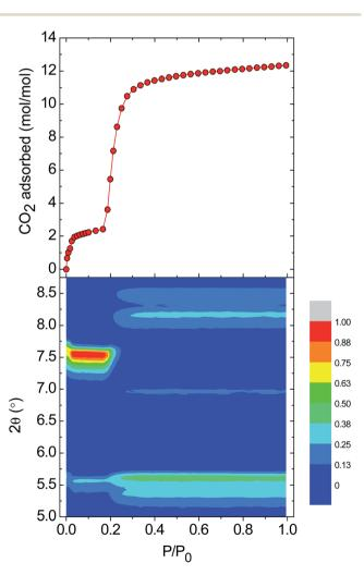
Fig. 4 (top) The adsorption branch of the CO<sub>2</sub> uptake measurements performed at 195 K on 1-a. (bottom) A contour plot of the evolution of the Bragg peaks over the range  $2\theta = 5.0-8.75^{\circ}$  as a function of  $P/P_0$ . The intensity of the peaks is relative to the strong peak observed at  $7.54^{\circ}$  over the pressure range  $P/P_0 = 0.035 - 0.18$ .
