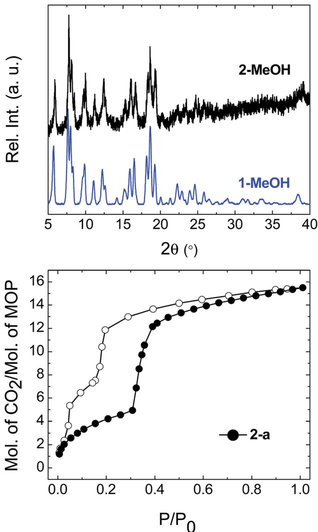
Fig. 7 (top) Comparison of the PXRD diffractograms for the flexible phase 1-MeOH and the phase obtained for the Rh-containing MOP 2-MeOH. (bottom) CO<sub>2</sub> sorption isotherms for 2-a, measured at 195 K. Filled circles represent adsorption and empty symbols desorption.
