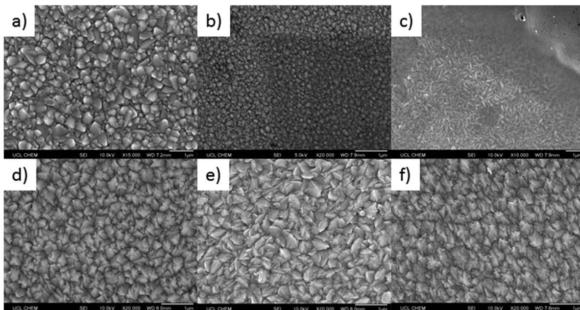
Fig. 3 Typical SEM images showing the surface morphology for (a) undoped  $\text{SnO}_2$ , (b) 0.1 mol% P: $\text{SnO}_2$ , (c) 0.25 mol% P: $\text{SnO}_2$ , (d) 0.5 mol% P: $\text{SnO}_2$ , (e) 1.0 mol% P: $\text{SnO}_2$ , and (f) 1.5 mol% P: $\text{SnO}_2$  thin films on glass. All samples were produced at 550 °C, by aerosol assisted CVD using compressed air as the carrier gas.
