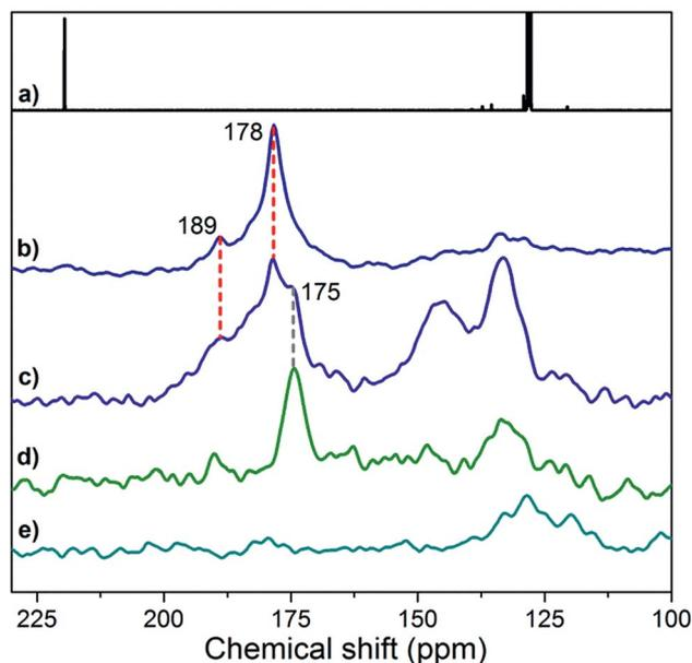
Fig. 3 (a)  $^{13}\text{C}$  NMR solution-state spectrum of free IMes\* ( $\text{C}_6\text{D}_6$ , 75 MHz); (b)  $^{13}\text{C}$  NMR solid-state HPDEC spectrum of  $2^*$  (30 000 scans);  $^{13}\text{C}$  NMR solid-state CP-MAS spectra of (c)  $2^*$  (90 000 scans), (d) IMes\*/ $\text{SiO}_2\text{-TMS}$  (27 513 scans) and (e)  $2^*$  (90 000 scans). Broader spectral windows are provided in Fig. S7 and S8† and  $^1\text{H}$  NMR spectra for IMes\* and  $2^*$  are given in Fig. S9.†
