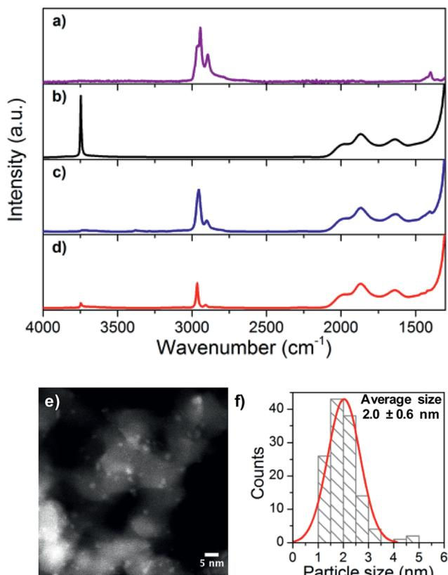
Fig. 1 FT-IR spectra of (a)  $[\text{Cu}_4(\text{HMDS})_4]$ , (b)  $\text{SiO}_{2-700}$ , (c)  $[\text{Cu}_4\text{HMDS}]/\text{SiO}_{2-\text{TMS}}$ , and (d)  $\text{Cu}/\text{SiO}_{2-\text{TMS}}$  (1) and (e) HR-TEM image and (f) particle size distribution of 1.
