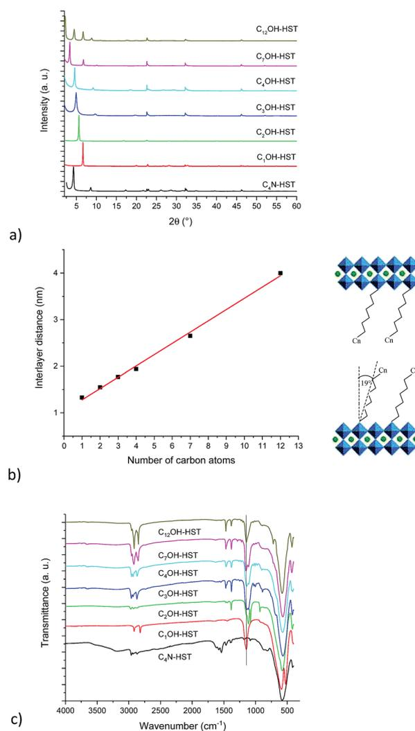
Fig. 1 (a) PXR patterns of the starting material **C<sub>4</sub>N-HST** and its reaction products with *n*-alcohols ( $\text{C}_n\text{OH}$ ,  $n = 1, 2, 3, 4, 7, 12$ ). (b) Left: Relationship between the number of carbon atoms in the aliphatic chain of *n*-alcohols and the interlayer distance of the corresponding grafted products (full line corresponds to the best linear fit). Right: Scheme of the bilayer arrangement of the mono-*n*-alkoxy-HST derivatives. (c) Corresponding IR spectra.
