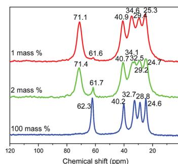
Fig. 9 Solid-state <sup>13</sup>C CP/MAS NMR spectra of the products resulting from the reaction between **HST** and 5-amino-pentan-1-ol with 1 mass% (red), 2 mass% (green) and 100 mass% (blue) of distilled water.
