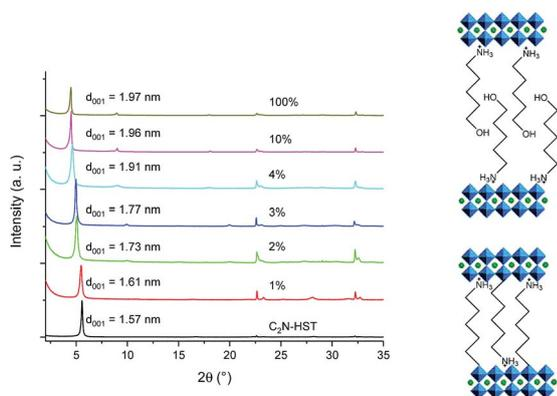
Fig. 8 Left: XRD patterns of **C<sub>2</sub>N-HST** and its reaction products with 5-amino-1-pentanol using different quantities of water. Right: Scheme of the pillaring arrangement (bottom), and of the bilayer arrangement (top).
