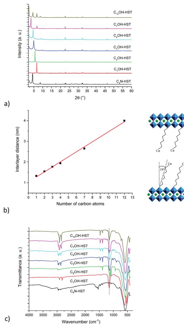
Fig. 1 (a) PXRD patterns of the starting material **C<sub>4</sub>N-HST** and its reaction products with *n*-alcohols ( $\text{C}_n\text{OH}$ ,  $n = 1, 2, 3, 4, 7, 12$ ). (b) Left: Relationship between the number of carbon atoms in the aliphatic chain of *n*-alcohols and the interlayer distance of the corresponding grafted products (full line corresponds to the best linear fit). Right: Scheme of the bilayer arrangement of the mono-*n*-alkoxy-HST derivatives. (c) Corresponding IR spectra.
