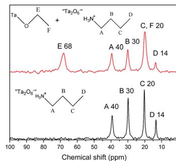
Fig. 7 Solid-state  $^{13}\text{C}$  CP/MAS NMR spectra of the products resulting from the reaction between **HST** and an equimolar mixture of butylamine and ethanol and 0.1 mass% (red) and 1 mass% (black) of distilled water.
