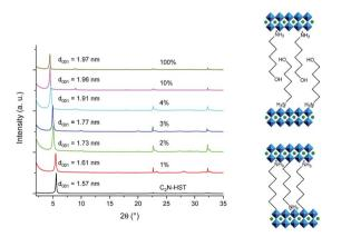
Fig. 8 Left: XRD patterns of C2N-HST and its reaction products with 5-amino-1-pentanol using different quantities of water. Right: Scheme of the pillaring arrangement (bottom), and of the bilayer arrangement (top).
