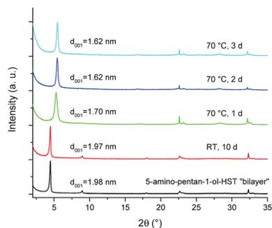
Fig. 10 XRD patterns of 5-amino-pentan-1-ol-HST "bilayer" and of the products obtained after heating.
