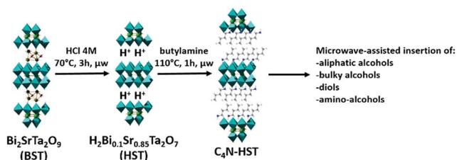
Scheme 1 Scheme of the general synthetic procedure.
