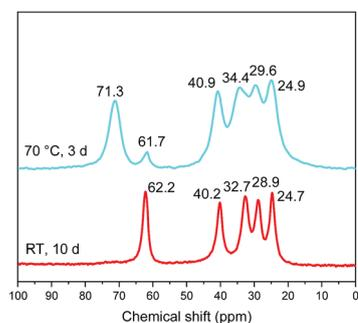
Fig. 11 Solid-state <sup>13</sup>C CP/MAS NMR spectra of **5-amino-pentan-1-ol-HST** "bilayer" (red) and the product obtained after heating (cyan).
