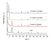
Fig. 6 PXRD patterns of HST and its reaction products with an equimolar mixture of butylamine and ethanol and 0 mass%, 0.1 mass% and 1 mass% of distilled water.
