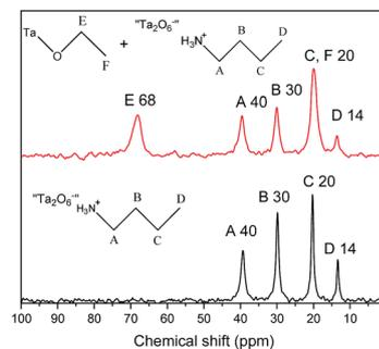
Fig. 7 Solid-state <sup>13</sup>C CP/MAS NMR spectra of the products resulting from the reaction between HST and an equimolar mixture of butylamine and ethanol and 0.1 mass% (red) and 1 mass% (black) of distilled water.
