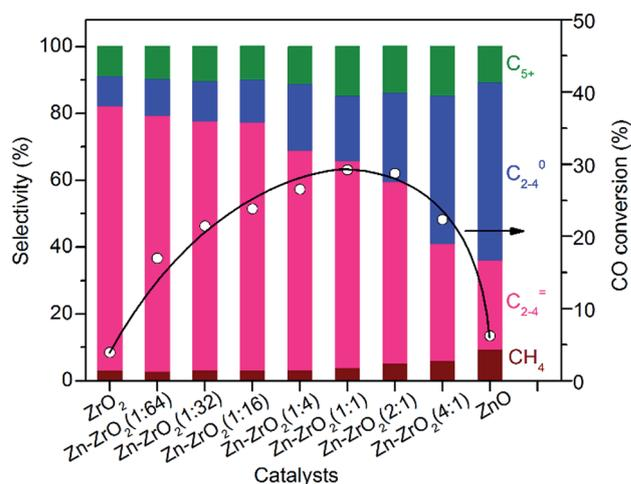
Fig. 3 Effect of Zn/Zr molar ratio on catalytic behaviours of the bifunctional Zn-ZrO<sub>2</sub>/H-SSZ-13-45H catalyst. The selectivity of CO<sub>2</sub> did not change with the ratio of Zn/Zr and was in the range of 41–45% for each catalyst. Reaction conditions: catalyst, 0.60 g;  $\text{H}_2/\text{CO} = 2$ ;  $P = 3 \text{ MPa}$ ;  $T = 673 \text{ K}$ ;  $F = 30 \text{ mL min}^{-1}$ ; time on stream, 10 h.
