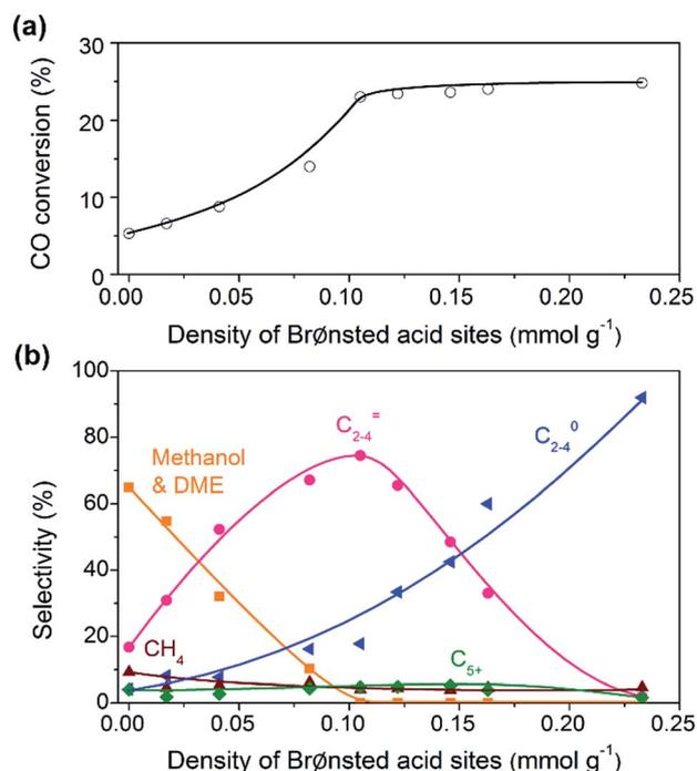
Fig. 5 Effect of density of Brønsted acid sites on catalytic behaviours of the bifunctional Zn-ZrO<sub>2</sub>/SSZ-13 catalyst. (a) CO conversion. (b) Product selectivity. The selectivity of CO<sub>2</sub> did not change with the density of Brønsted acid sites and was in the range of 41–45%. Reaction conditions: catalyst, 0.60 g; H<sub>2</sub>/CO = 2; P = 3 MPa; T = 673 K; F = 30 mL min<sup>-1</sup>; time on stream, 10 h.
