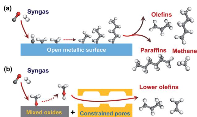
Fig. 1 Illustration of two types of direct conversion of syngas into lower olefins. (a) FT-synthesis route on a Fe-based catalyst. (b) SMO (syngas *via* methanol intermediate to olefin) route on one bifunctional catalyst.
