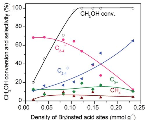
Fig. 11 Effect of density of Brønsted acid sites for the conversion of methanol over SSZ-13 zeolites. Reaction conditions: catalyst, 0.4 g;  $F(\text{H}_2) = 30$  mL min<sup>-1</sup>;  $F(\text{liquid CH}_3\text{OH}) = 0.01$  mL min<sup>-1</sup>;  $P = 2$  MPa;  $T = 673$  K; time on stream, 3 h.
