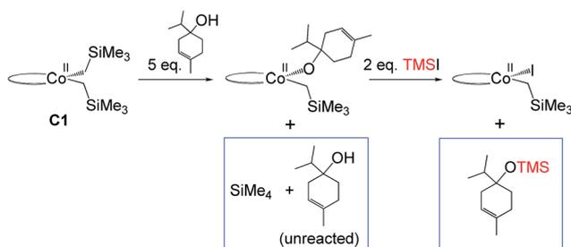
Fig. 9 Indirect evidence for formation of an alkoxide intermediate. Components in boxes were identified *via* NMR (see ESI<sup>†</sup>).
