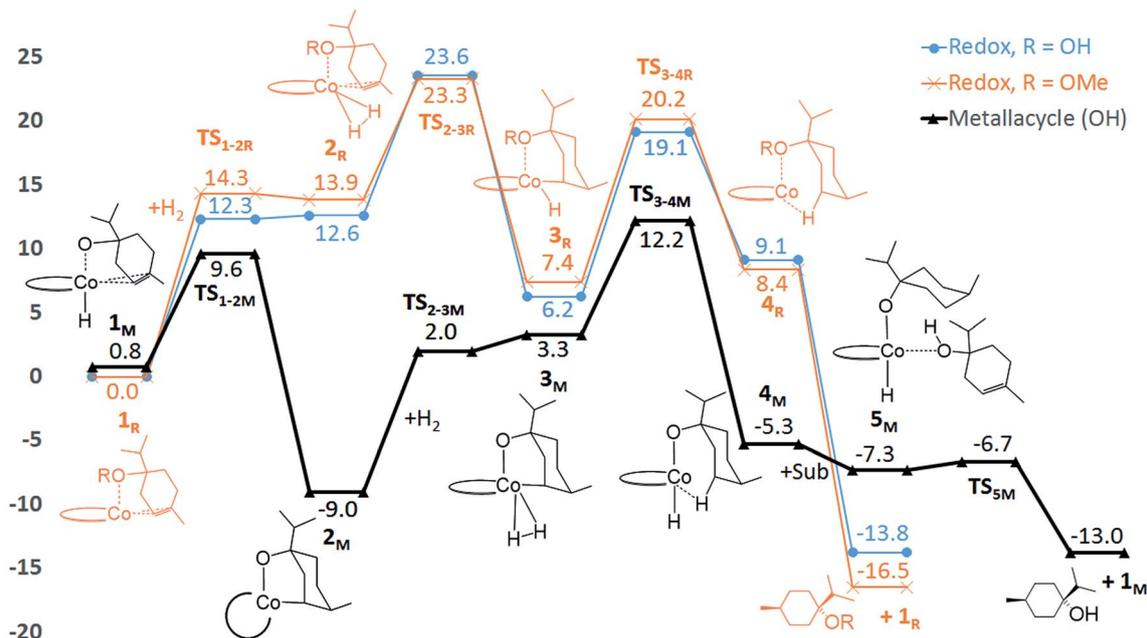
Fig. 4 Computed free energies ( $\text{kcal mol}^{-1}$ ) for C1-catalysed hydrogenation. The redox mechanism is shown for substrates terpinen-4-ol ( $R = \text{OH}$ , blue line) and its methoxy derivative ( $R = \text{OMe}$ , orange line). The metallacycle mechanism is shown for terpinen-4-ol (black line). All energies are referenced to the  $1_R$  state of each substrate.
