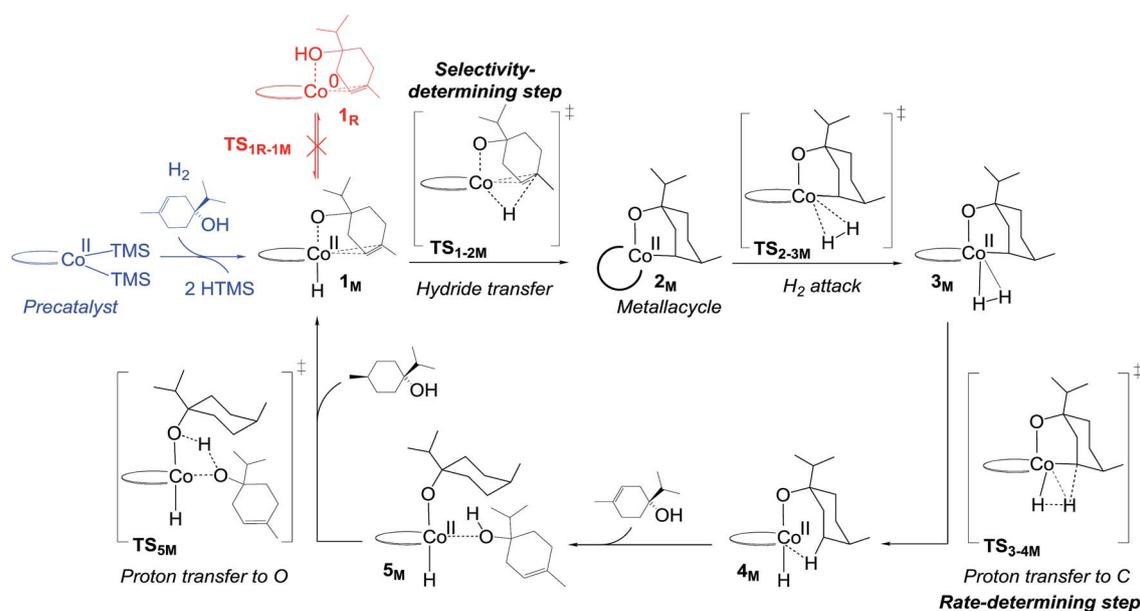
Fig. 5 Non-redox metallacycle mechanism proposed for bis(phosphine)cobalt-catalysed hydrogenation of terpinen-4-ol. For details on the activation of the precatalyst, see Fig. S5, ESI<sup>†</sup>.
