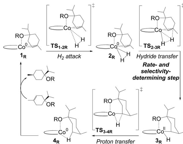
Fig. 3 Co(0)–Co(II) redox mechanism computed for C1-catalysed hydrogenation of terpinen-4-ol (R = H) and its methoxy-derivative (R = CH<sub>3</sub>). Computed energies are shown in Fig. 4. Terpinen-4-ol prefers an alternative mechanism, Fig. 5.
