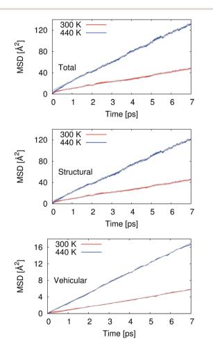
Fig. 1 Mean-squared displacements (MSD) as functions of time for the proton at 300 and 440 K. The gray lines represent the linear regression used for extraction of the diffusion coefficients. The linear regression was performed on the data between 1 and 7 ps. The top panel gives the total MSD, while the middle and bottom panels show the structural and vehicular components, respectively.
