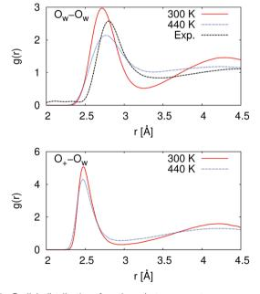
Fig. 2 Radial distribution functions between water oxygen atoms  $(O_W-O_W)$  and between the hydronium ion oxygen atom and the water oxygen atoms  $(O_+-O_W)$ . At 300 K, the simulated water is over-structured compared to the experimental reference. While at 440 K, the simulated water is now under-structured compared to the experimental reference is from Skinner et al., <sup>36</sup> and we note that the experimental reference is for pure water while our simulations are for  $\sim 1.7$  M HCl.
