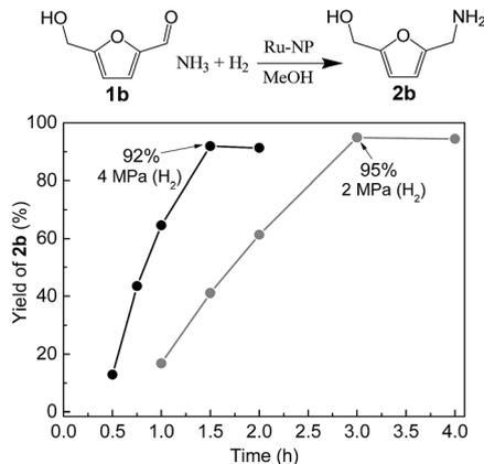
Fig. 5 Time courses of reductive amination of 5-hydroxymethylfurfural (**1b**) over Ru-NP. Reaction conditions: catalyst (0.2 mg), **1b** (0.5 mmol), MeOH (5 mL), NH<sub>3</sub> (8 mmol), and H<sub>2</sub> (2 and 4 MPa), 363 K.
