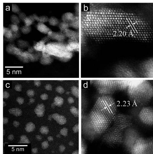
Fig. 1 (a) HAADF-STEM and (b) high magnification HAADF-STEM images of Ru-NPs prepared from 10 wt% Ru-deposited  $\text{Ca}(\text{NH}_2)_2$ . (c) HAADF-STEM and (d) high magnification HAADF-STEM images of 10 wt% Ru/ $\text{Ca}(\text{NH}_2)_2$ .
