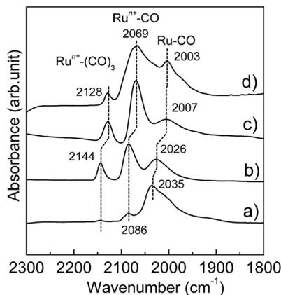
Fig. 4 Difference DRIFT spectra for adsorption of CO onto (a) Ru-NP, (b) Ru/Nb<sub>2</sub>O<sub>5</sub>, (c) Ru/SiO<sub>2</sub> and (d) Ru-HCP samples at 103 K.
