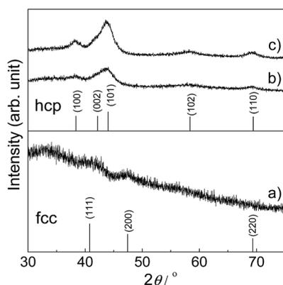
Fig. 2 XRD patterns of Ru-NP samples prepared from (a) 10 wt%, (b) 15 wt% and (c) 20 wt% Ru-deposited Ca(NH<sub>2</sub>)<sub>2</sub>. JCPDF card numbers are (hcp) 01-070-0274 and (fcc) 01-088-2333.
