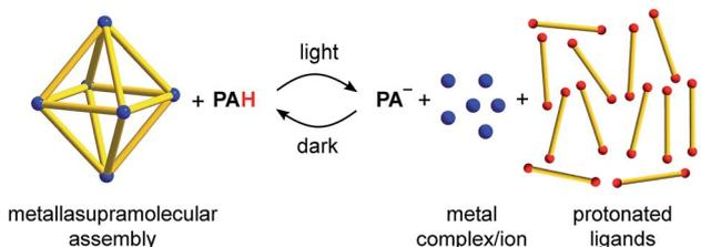
**Scheme 1** Reversible disassembly of metallasupramolecular structures by means of a metastable-state photoacid (**PAH**). The M<sub>6</sub>L<sub>12</sub> coordination cage is used as a representative example of a metal–ligand assembly.
