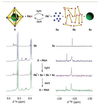
Scheme 4 Irradiation of a mixture of cage 5 (10  $\mu$ M), NaCl (60  $\mu$ M), and the photoacid PAH (8 equiv. with respect to each bipyridyl ligand) in CD<sub>3</sub>CN/D<sub>2</sub>O (8 : 2) by violet light results in disassembly of the cage and liberation of the [B(p-C<sub>6</sub>H<sub>4</sub>F)<sub>4</sub>]<sup>-</sup> guest (green ball) as evidenced by the <sup>1</sup>H NMR (left) and <sup>19</sup>F NMR spectra (right). Details about the bridging ligand (yellow) are given in the ESI.†
