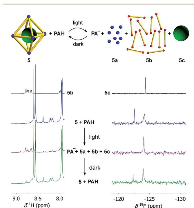
Scheme 4 Irradiation of a mixture of cage **5** (10  $\mu M$ ), NaCl (60  $\mu M$ ), and the photoacid PAH (8 equiv. with respect to each bipyridyl ligand) in  $CD_3CN/D_2O$  (8 : 2) by violet light results in disassembly of the cage and liberation of the  $[B(p-C_6H_4F)_4]^-$  guest (green ball) as evidenced by the  $^1H$  NMR (left) and  $^{19}F$  NMR spectra (right). Details about the bridging ligand (yellow) are given in the ESI.†
