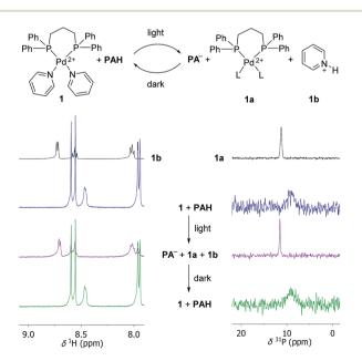
Scheme 3 Irradiation of a mixture of complex 1 (125 µM) and the photoacid PAH (8 equiv.) in CD<sub>3</sub>CN/D<sub>2</sub>O (8 : 2) by violet light results in the displacement of the pyridyl ligands as evidenced by the <sup>1</sup>H NMR (left side) and <sup>31</sup>P NMR spectra (right side). The triflate anions of 1 are not shown for clarity. L indicates solvent or OTf-.
