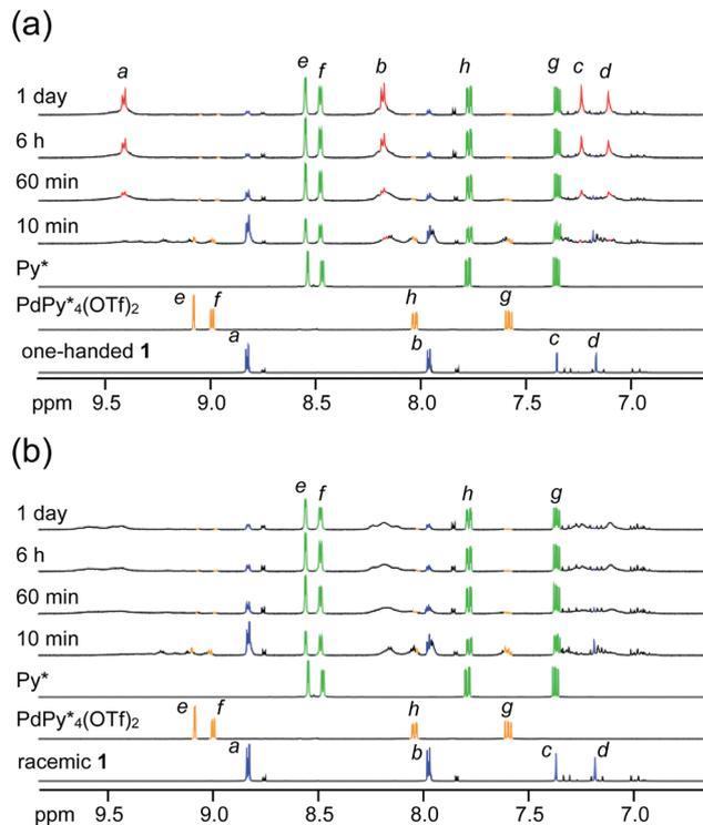
Fig. 2 Partial  $^1\text{H}$  NMR spectra (500 MHz, aromatic region,  $\text{CD}_3\text{NO}_2$  and  $\text{CD}_2\text{Cl}_2$  (v/v = 4/1), 298 K) of the reaction mixture of the self-assembly of the homochiral  $\text{Pd}_6\text{1}_8$  capsule(s) from  $\text{PdPy}_4^*(\text{OTf})_2$  and (a) one-handed  $\mathbf{1}^*$  ( $[\mathbf{1}^*]_0 = 2.2 \text{ mM}$ ) and (b) a racemic mixture of  $\mathbf{1}$  ( $[\mathbf{1}]_0 = 2.2 \text{ mM}$ ). The lettering refers to that shown in Fig. 1.
