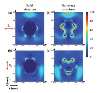
Fig. 2 Calculated electric field distributions ( $|E|^2/|E_0|^2$ ) for (a) and (b) the solid Ag–Au octahedron and (c) and (d) the hollow Ag–Au SAMCs. The red arrows in the figure show the polarization directions of the incident light.
