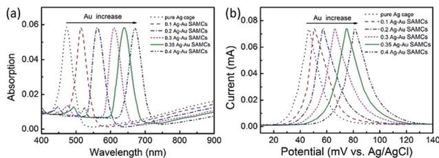
Fig. 3 (a) UV-vis spectra and (b) LSV curves of the as-synthesized Ag–Au SAMCs with different Au content. LSV measurements: 1 M KCl electrolyte, scan rate of 5 mV s<sup>-1</sup>.
