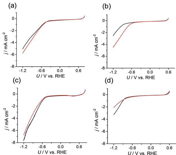
Fig. 2 Current density ( $j$ ) versus potential ( $U$ ) curves obtained from (a) Co-CTF, (b) Ni-CTF, (c) Cu-CTF, and (d) CTF in a phosphate buffer (saturated with Ar, black line) and a KHCO<sub>3</sub> electrolyte (saturated with CO<sub>2</sub>, red line).
