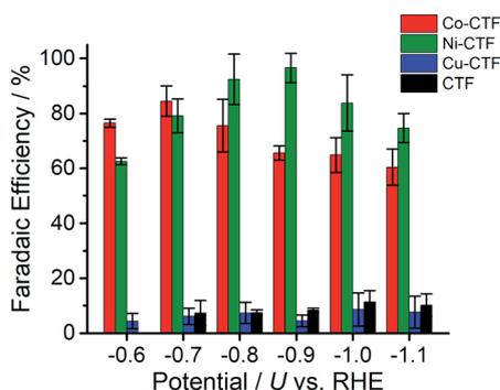
Fig. 3 Effect of potential on the faradaic efficiency values during the CO<sub>2</sub>RR to generate CO using Co-CTF (red), Ni-CTF (green), Cu-CTF (blue) and CTF (black) in a KHCO<sub>3</sub> electrolyte (saturated with CO<sub>2</sub>) at pH 6.8. The error bar represents the standard deviation from three experimental trial.
