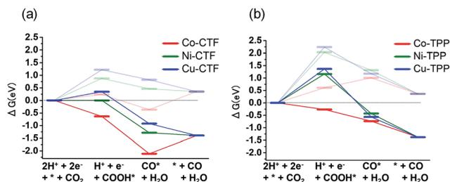
Fig. 5 Free energy diagrams for CO<sub>2</sub> reduction to CO on Co (red), Ni (green) and Cu (blue)-modified (a) CTF, and (b) TPP at 0 V (pale lines) and -0.87 V (dark lines).
