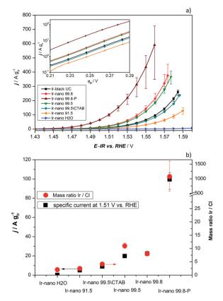
Fig. 5 (a) OER activity of all compared catalysts. The scanning rate, temperature and rotation speed are 5 mV s $^{-1}$ , 25 °C, and 2300 rpm, respectively. The measurements were performed in 0.5 M  $\rm H_2SO_4$  and Ar-saturated solution; the inset shows the data as Tafel plots; (b) specific current density at 1.51 V vs. RHE measured under the same experimental conditions. The right axis indicates the Ir/Cl mass ratio recorded by EDX.
