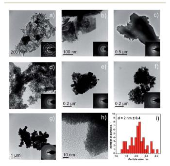
Fig. 3 TEM images of catalysts (a) Ir-black; (b) Ir-nano H<sub>2</sub>O; (c) Ir-nano 91.5; (d) Ir-nano 99.5\CTAB; (e) Ir-nano 99.5; (f) Ir-nano 99.8; and (g), (h) Ir-nano 99.8-P; the insets show the electron diffraction pattern from the synthesized materials showing the (111), (002), (022), (311), and (222) reflections of metallic Ir. (i) Histogram of Ir-nano 99.8-P.
