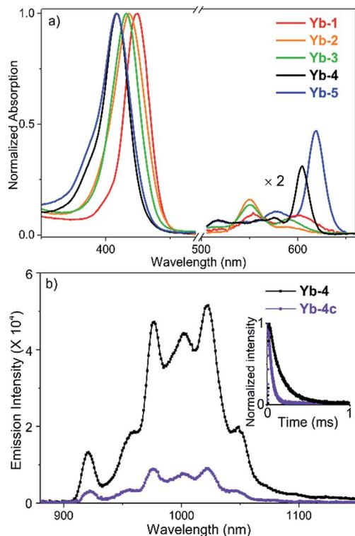
Fig. 1 (a) Normalized absorption spectra of Yb-1–5 in water with 0.1% DMSO; (b) emission spectra of Yb-4 and Yb-4c in water (0.1% DMSO,  $\lambda_{\text{ex}} = 410$  nm,  $A_{410\text{nm}} = 0.1$ ). Inset: decay curves of Yb-4 and Yb-4c in water monitored at 980 nm.
