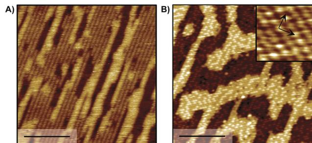
Fig. 3 STM images of (A) 0.06 ML and (B) 0.19 ML trifluoroacetate on Au(110) demonstrate that carboxylates form dense local island at low global coverages; scale bar, 10 nm, sample bias: 0.5–1.5 V, tunneling current: 0.1 nA. Inset in B reveals the  $c(2 \times 2)$  ( $\sim 400$  K annealed surface in B).
