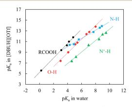
Fig. 4 Correlations between  $pK_as$  of N-H ( $\blacksquare$ ), N<sup>+</sup>-H ( $\blacktriangle$ ), O-H ( $\spadesuit$ ), and carboxylic (RCOOH,  $\blacksquare$ ) acids in [DBUH][OTf] and those in water; the linearity ( $R^2$ ) of each individual correlation is better than 0.991 (ESI†). The ESI provides further details of the acidity correlation equations between these two solvents (eqn S3-6†).
