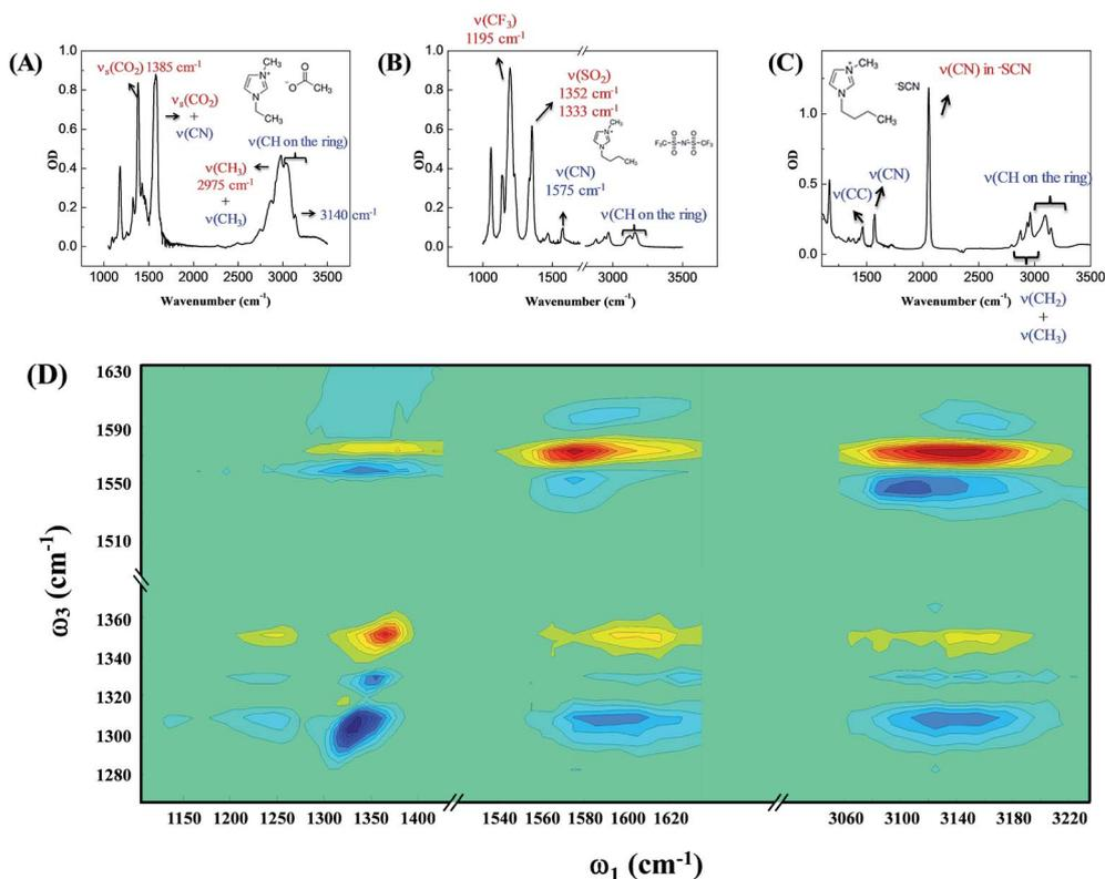
Fig. 1 FTIR spectra of (A) 1-ethyl-3-methylimidazolium acetate; (B) 1-butyl-3-methylimidazolium bis(trifluoromethylsulfonyl)imide; (C) 1-butyl-3-methylimidazolium thiocyanate. The peaks were assigned based on comparison with *ab initio* calculations and database results. (D) 2D IR spectrum of 1-butyl-3-methylimidazolium bis(trifluoromethylsulfonyl)imide at time zero.
