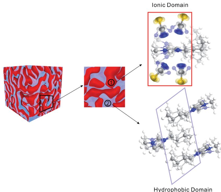
**Scheme 1** Schematic of structures of ILs. On the mesoscale, ILs form a bicontinuous structure, comprised of ionic domains and hydrophobic domains. In the ionic domain, the interionic orientation is random.
